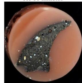
Fig. 2e. Results of the copper droplets coagulation after the St1, St2, R2 (5% of each), and St4 (2%) - chemical treatment performed for 10 minutes
