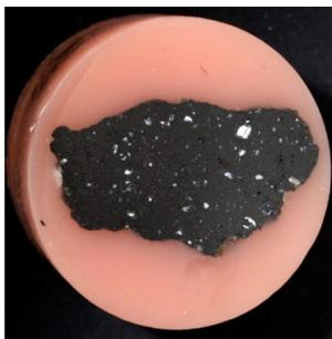
Fig. 2h. Results of the copper droplets coagulation after the R1 (5%) - chemical treatment performed for 20 minutes
