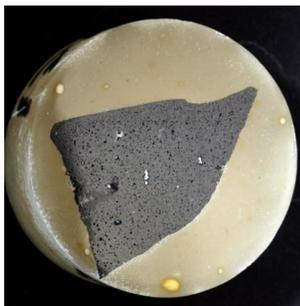
Fig. 2g. Results of the copper droplets coagulation without the chemicals treatment performed for 20 minutes
