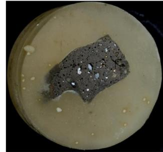
Fig. 2h. Results of the copper droplets coagulation after the R2, R3, St1, St2, St3 (5% of each), and St4 (2%) - chemical treatment performed for 20 minutes
