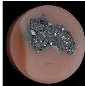
Fig. 2c. Results of the copper droplets coagulation after the St1, St2, and R2 (5% of each) - chemicals treatment performed for 10 minutes
