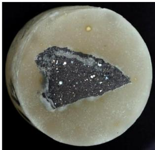
Fig. 2a. Results of the copper droplets coagulation after the St1 (5%) - chemical treatment performed for 10 minutes
