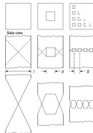
Fig. 7. Simple ductile failure model [2]
