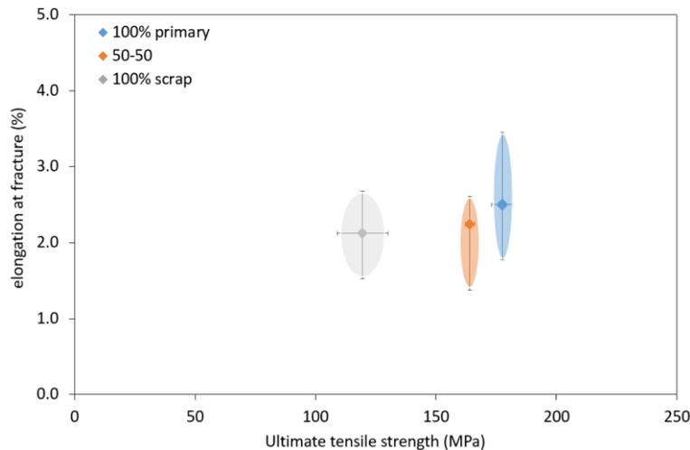
Fig. 5. Bubble diagram of the tensile test results
