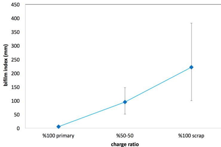
Fig. 4. Bifilm index of different charges
