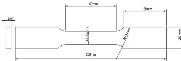
Fig. 1. Sizes and shape of tensile specimen
