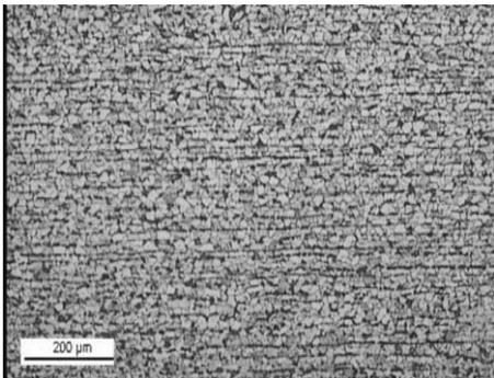
Fig. 3. Microstructure of the base metal, ferrite phase is bright and perlite phase is dark, optical microscopes of Dewinter Company
