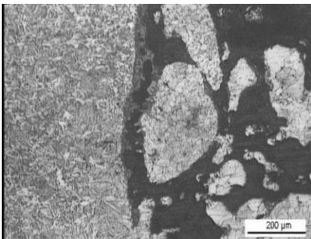
Fig. 7. Repaired specimen with the groove width size of 1mm, metallurgical defects in the dark color in the repaired place, optical microscope of Dewinter Company
