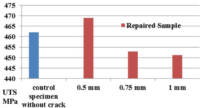
Fig. 4. Comparison of tensile strength of control specimen and repaired specimens
