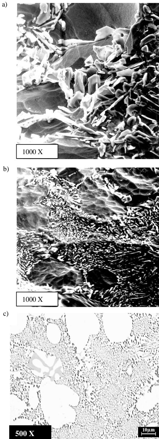
Fig. 2. Microstructures of the alloy AK11: a – refined alloy, b – refined and modified alloy, c – refined, modified and filtrated alloy
