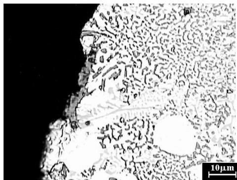
Fig. 4. Microstructures of the filters cast with the alloy AK11: a- form and distribution of impurities in the casted filter, b –retention of the impurity in the refined alloy, c – retained impurities and the secondary phases which occurred in the modified alloy
