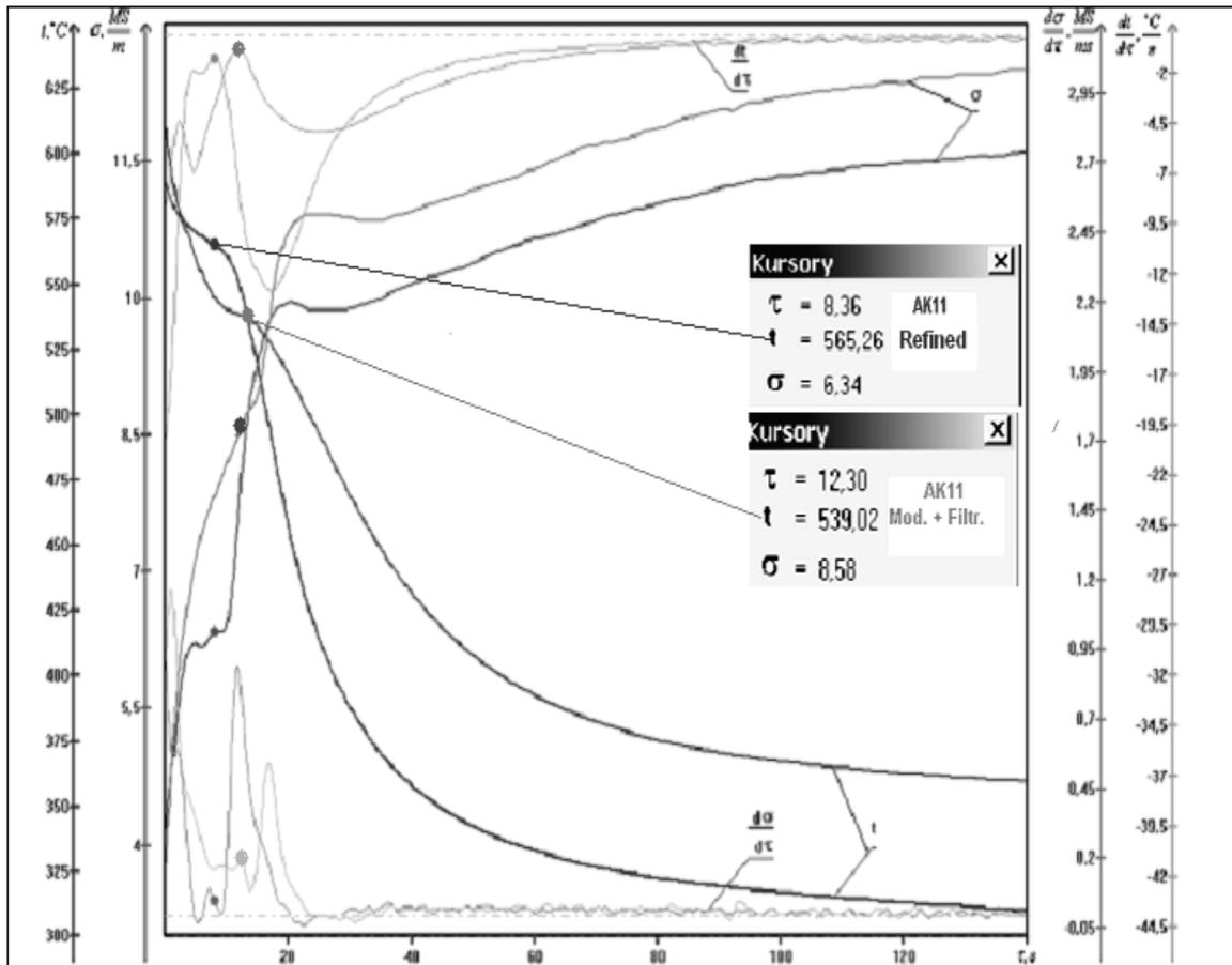
Fig. 1. Graphic record of the crystallization curves for the alloy AK11 after carried out metallurgical operations
