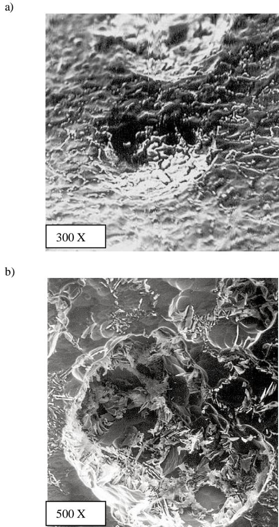
Fig. 3. Internal defects in the microstructure of the alloy AK11, cast directly from the pig sows: a – gaseous porosity (bubbles), b – gaseous – shrinkage porosity and the oxide film
