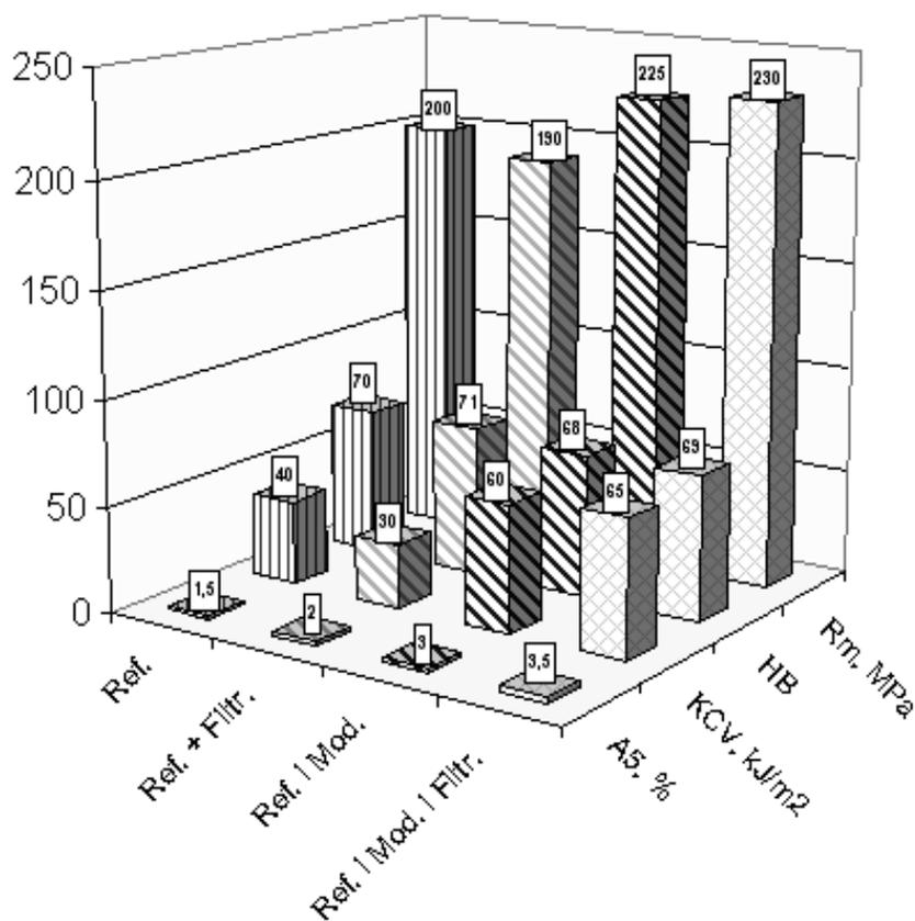
Fig. 5. Comparison of the mechanical properties for the alloy AK11
