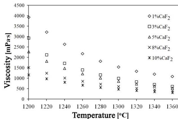
Fig. 5. Influence of added CaF<sub>2</sub> on viscosity of decopperised slag
