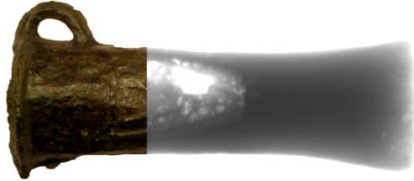
Fig. 9. X-ray image of axe No. NG15 together with the view of part of the artefact with visible defects
