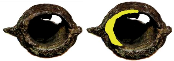
Fig. 5. Axe, visible remains of gating systems – marked in yellow (axe No. NG25)
