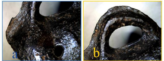
Fig. 6. Axe (No. NG7) with remained elements of the gating system and casting defects: incomplete filling - misrun (a) and flashes along the line joining the mould (b)
