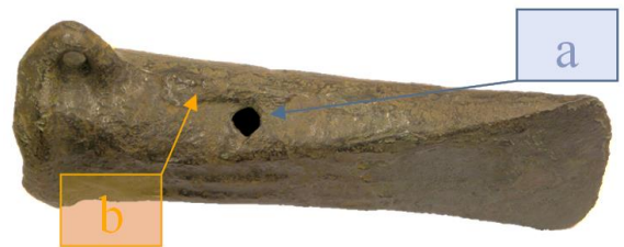
Fig. 6. Axe (No. NG7) with remained elements of the gating system and casting defects: incomplete filling - misrun (a) and flashes along the line joining the mould (b)
