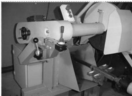
Fig 2. Abrasive cut-off machine- general view
