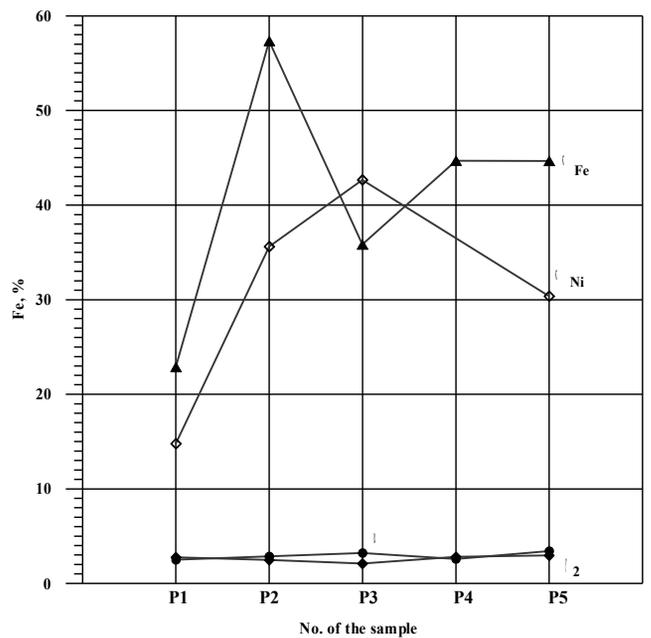
Fig. 8. The concentration Fe in the phases of the bronze P1-P5:  $\alpha$ ,  $\gamma_2$ ,  $\kappa_{Fe}$ ,  $\kappa_{Ni}$
