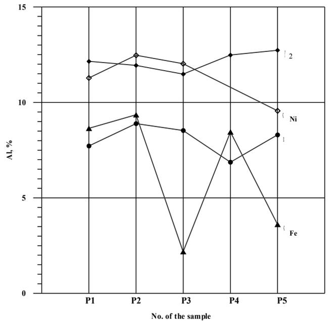
Fig. 7. The concentration Al in the phases of the bronze P1-P5:  $\alpha$ ,  $\gamma_2$ ,  $\kappa_{Fe}$ ,  $\kappa_{Ni}$
