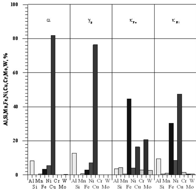
Fig. 5. The concentration of elements in the phases of the bronze CuAl10Fe5Ni5CrSiMoW (P5):  $\alpha$ ,  $\gamma_2$ ,  $\kappa_{Fe}$ ,  $\kappa_{Ni}$
