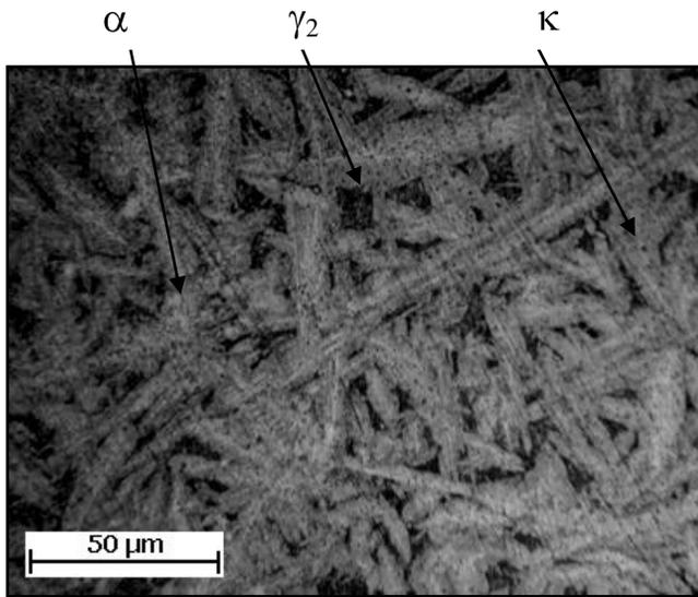
Fig. 17. The microstructure of the bronze CuAl10Fe5Ni5MoSi
