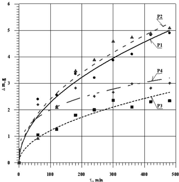
Fig. 20. The abrasive wear of the bronze CuAl10Fe5Ni5Si (P1) with additions Cr (P2), Mo (P3) and W (P4)
