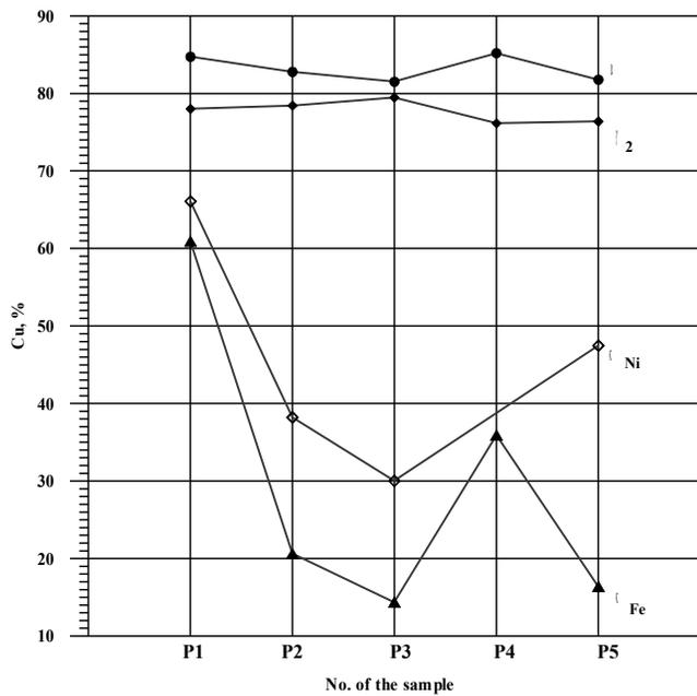
Fig. 6. The concentration Cu in the phases of the bronze P1-P5:  $\alpha$ ,  $\gamma_2$ ,  $\kappa_{Fe}$ ,  $\kappa_{Ni}$
