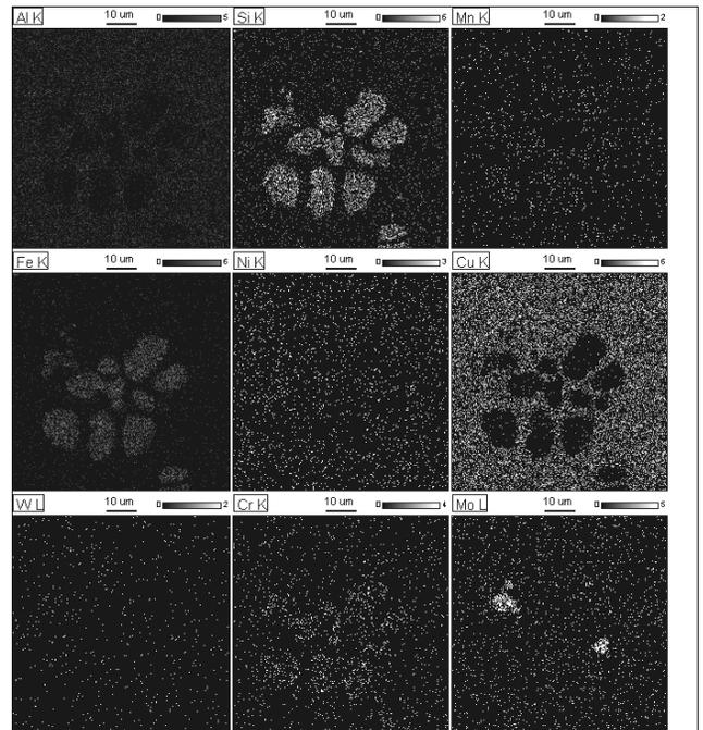
Fig. 4. The map of the surface distribution of elements in the microstructure of the bronze CuAl10Fe5Ni5CrSiMoW
