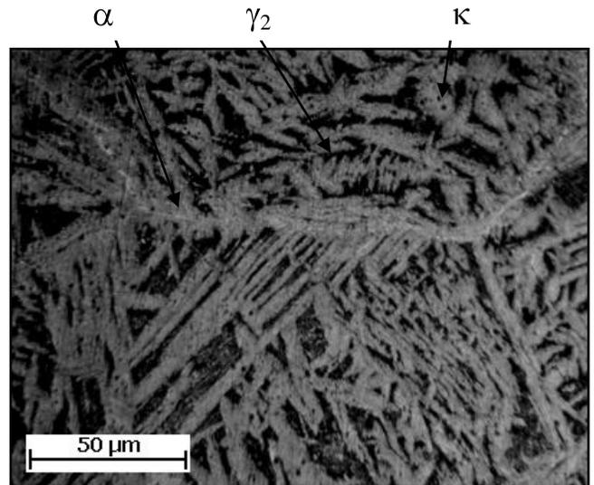
Fig. 16. The microstructure of the bronze CuAl10Fe5Ni5CrSi
