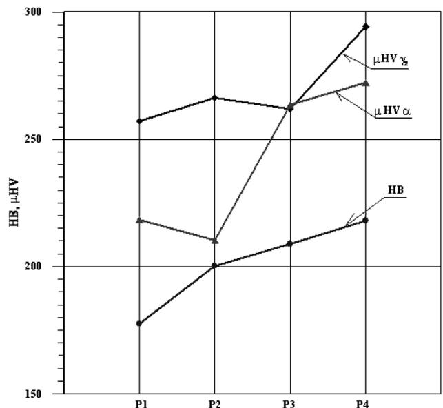
Fig. 19. The hardness HB of the bronze and the  $\mu\text{HV}$  of the phase  $\alpha$  and  $\gamma_2$
