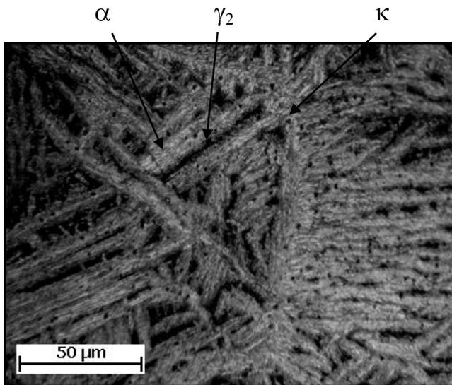
Fig. 18. The microstructure of the bronze CuAl10Fe5Ni5SiW
