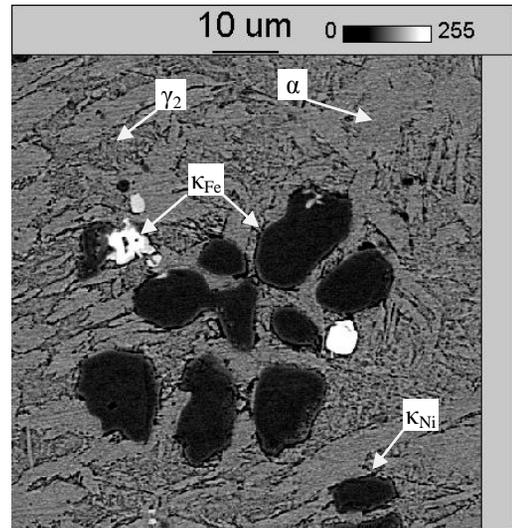
Fig. 3. The microstructure of the bronze CuAl10Fe5Ni5CrSiMoW
