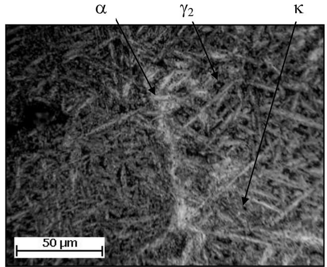
Fig. 15. The microstructure of the bronze CuAl10Fe5Ni5Si
