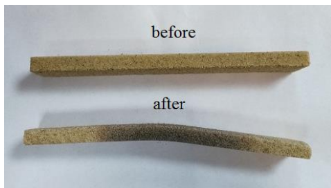
Fig. 1. Deformation of moulding sand with the geopolymer binder Geopol ® during hot-distortion tests [33]
