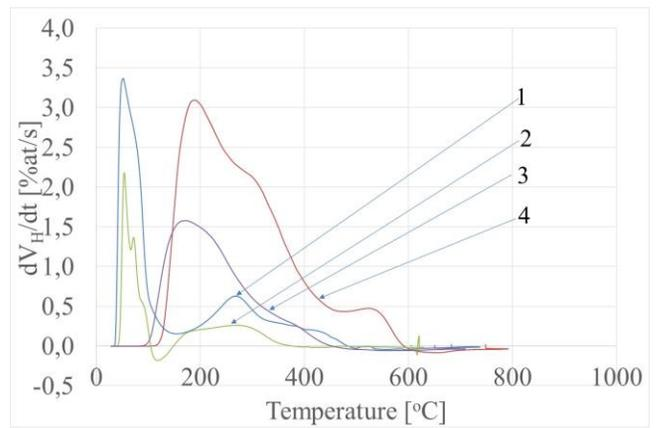
Fig. 7. Changes in hydrogen content in gases evolved during casting of ductile iron related to the mould temperature: 1) casting thickness 13 mm, sand with the SL resin, 2) casting thickness 13 mm, sand with the SL 2002 resin, 3) casting thickness 40 mm, sand with the SL resin, 4) casting thickness 40 mm, sand with the SL 2002 resin
