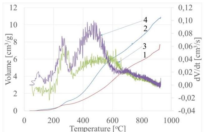
Fig. 10 Gas forming tendency and its changes observed in the sand with: 1) SL resin, 2) SL2002 resin, 3) SL resin (instantaneous values), 4) SL2002 resin (instantaneous values)
