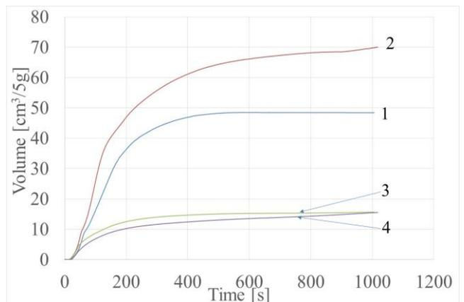
Fig. 9. Gas volume released during heating up 5 grams of the sand with: 1) SL resin, 2) SL2002 resin, 3) SL resin (reheating), 4) SL2002 resin (reheating)
