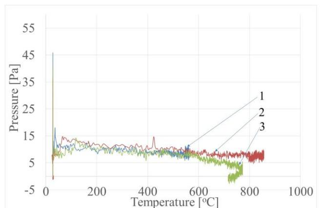
Fig. 4. Pressure of gases released from mould with the SL2002 resin during pouring of ductile iron castings with the wall thickness: 1) 13 mm, 2) 26 mm, 3) 40 mm
