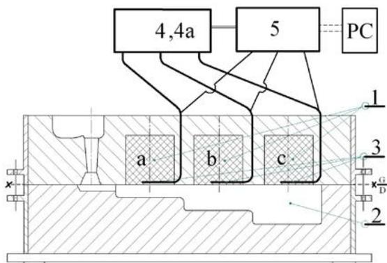
Fig. 1. Test stand for direct measurement of gas evolution from moulding sands: 1) mould elements (height of mould cavity under the measuring point: a-13 mm, b-26 mm, c-40 mm), 2) mould cavity with the gating system, 3) gas sampling location, 4) and 4a) gas sensors, 5) Agilent recorder [8, 9]
