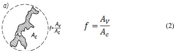
Fig. 4. Scheme of shapes of graphite precipitates cross-sections [12]
