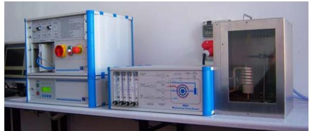
Fig. 1. UMSA device used for the thermal derivative analysis
