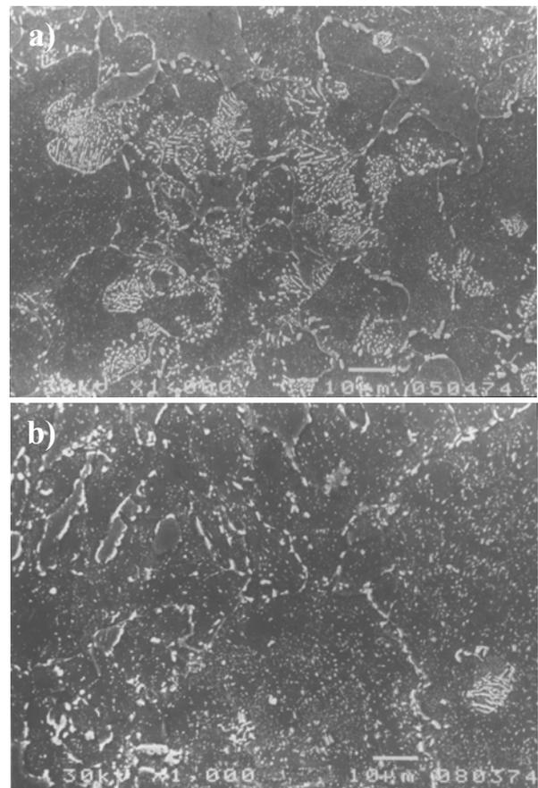
Fig. 1. Structure of the cast steel after service: a) G21; b) G17
