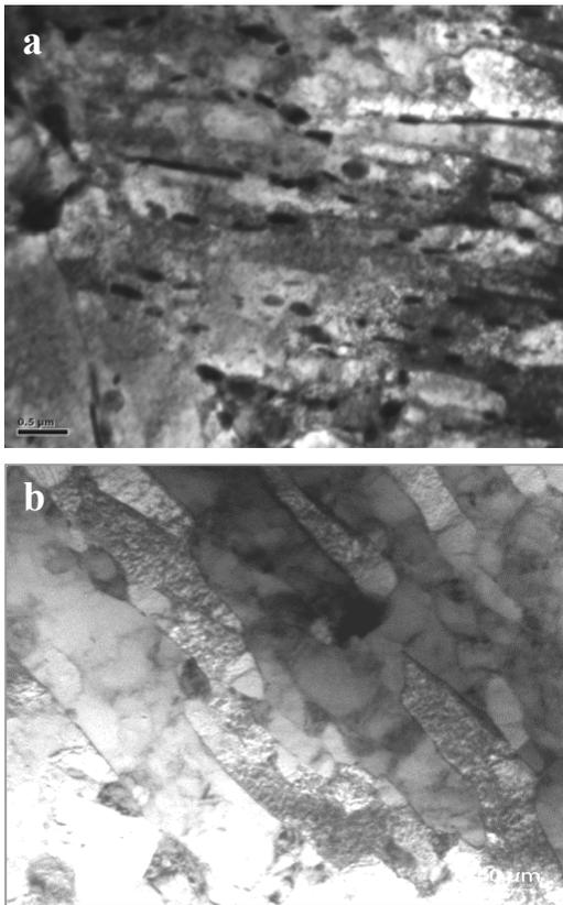
Fig. 2. Structure of the investigated cast steels after bainitic hardening and tempering: a) G21 and b) G17
