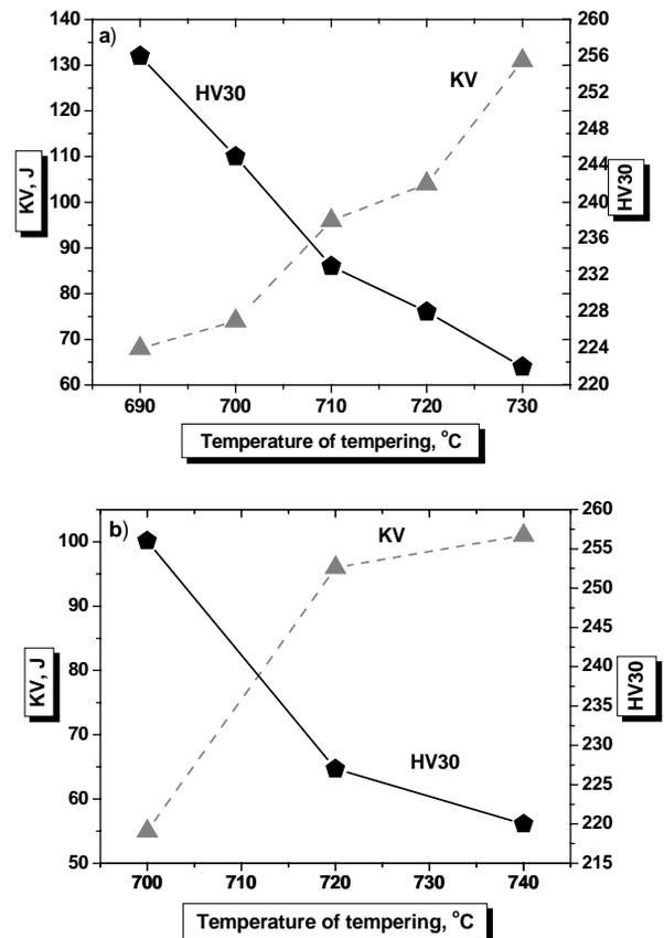
Fig. 3. Influence of the tempering temperatures on cast steels properties: a) G21; b) G17
