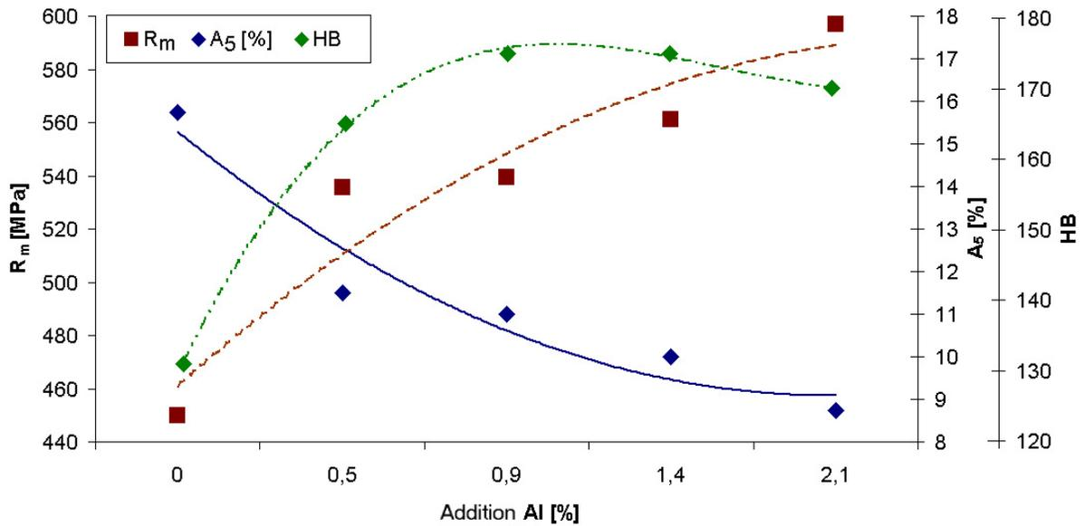
Fig. 1. Influence of aluminium addition on mechanical properties ( $R_m$ ,  $A_5$  and HB) of brass CuZn40Ni6
