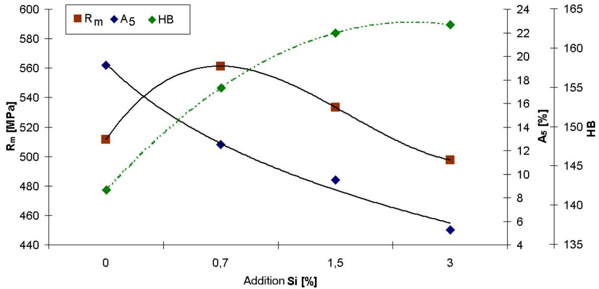
Fig. 3. Influence of additions of silicon on mechanical properties ( $R_m$ ,  $A_5$  and HB) of brass CuZn41Ni6
