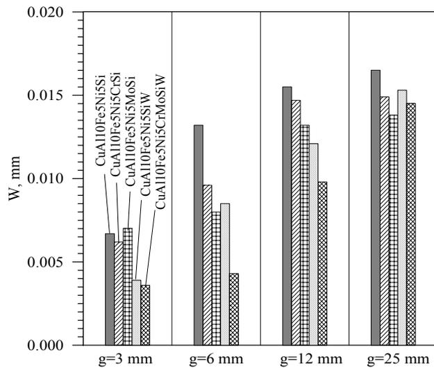
Fig. 7. The value the average width  $W$  the separates of the phase  $\alpha$  on the boundary of the primitive phase  $\beta$
