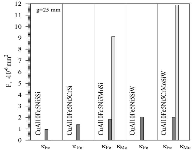
Fig. 8. The average value of the field  $F$  of the surface of phases  $\kappa$
