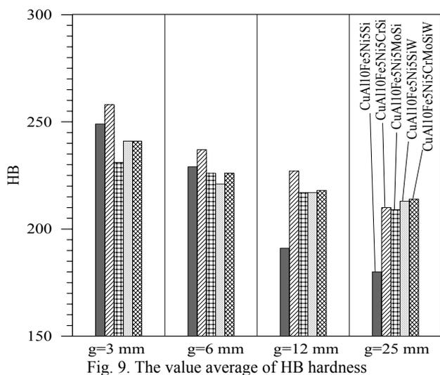
The difference was introduced on the figure 3  $\Delta$ HB among the average hardness HB of the wall of the test cast of studied bronzes about the thickness 3 mm and 25 mm.
