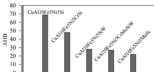
Fig. 10. Range of fall of hardness HB on thickness of wall of cast from 3 mm to 25 mm
