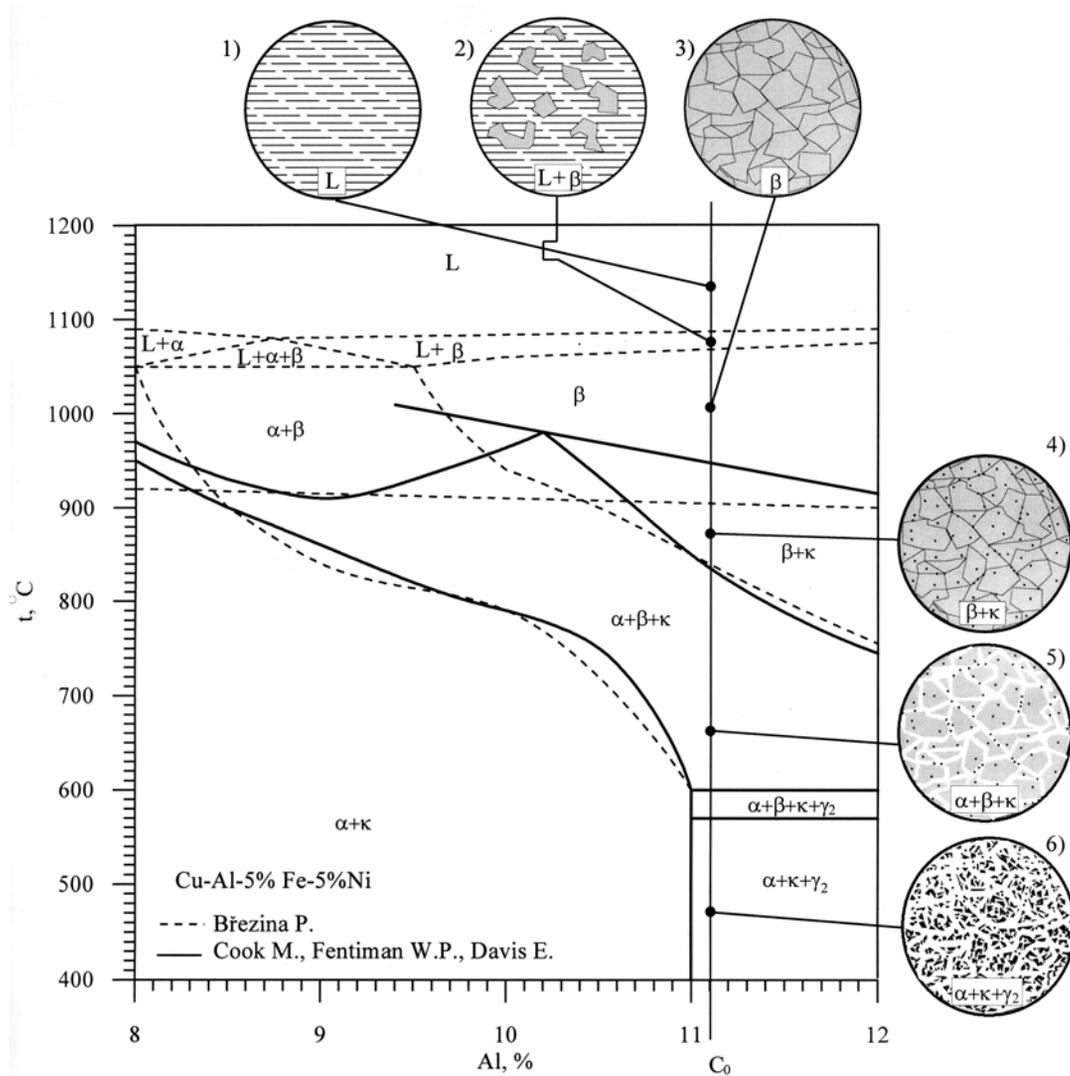
Fig. 2. The model of the crystallization of the bronze with the concentration  $C_0$
