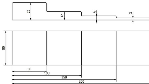
Fig. 1. The pattern of test cast with the changing thickness of the wall
