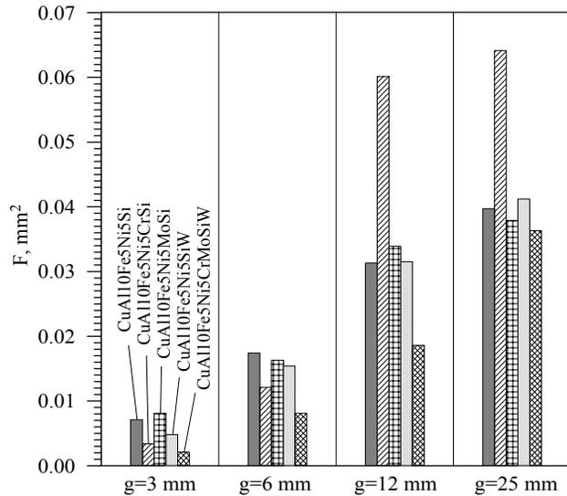
Fig. 6. The average value of the field  $F$  of the surface of the primary phase  $\beta$
