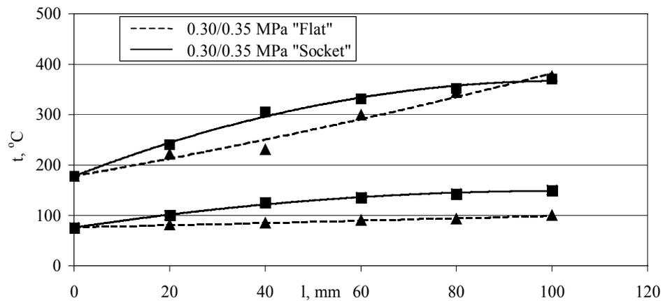
Fig. 9. Effect of distance from cooling nozzle axis and cooling time on temperature of casting die with flat heat transfer surface („Flat”) and surface with cylindrical socket („Socket”) cooling with water mist under pressure 0.30/0.35 MPa
