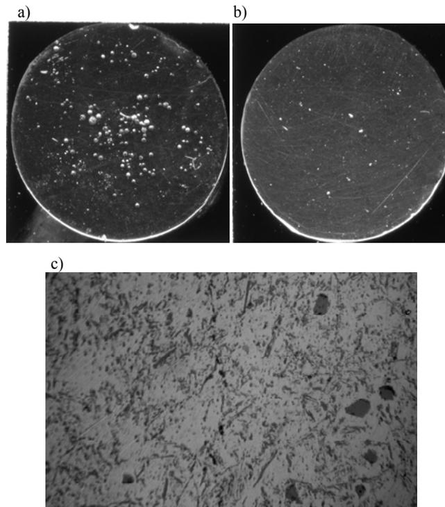
Fig. 10. Porosity of uncooled (a) and of cooled casting (b) and microstructure (c) of cooled with water mist under pressure 0.40/0.45 MPa; magnification: a), b) x 4, c) x 200
