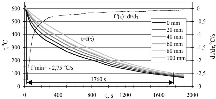
Fig. 4. Effect of time and distance from cooling nozzle axis on temperature and cooling rate with air under pressure 0.40 MPa of casting die with flat heat transfer surface
