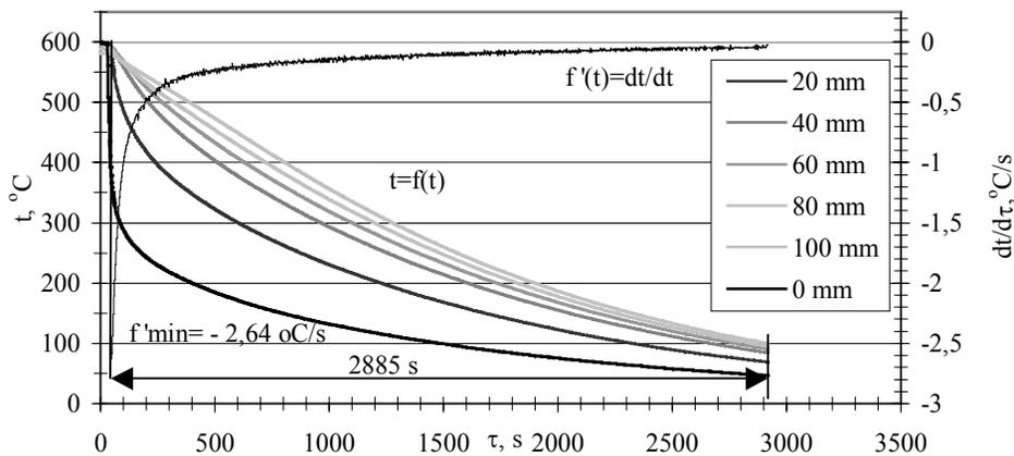
Fig. 6. Effect of time and distance from cooling nozzle axis on temperature and cooling rate with water mist under pressure 0.30/0.35 MPa of casting die with cylindrical socket in heat transfer surface
