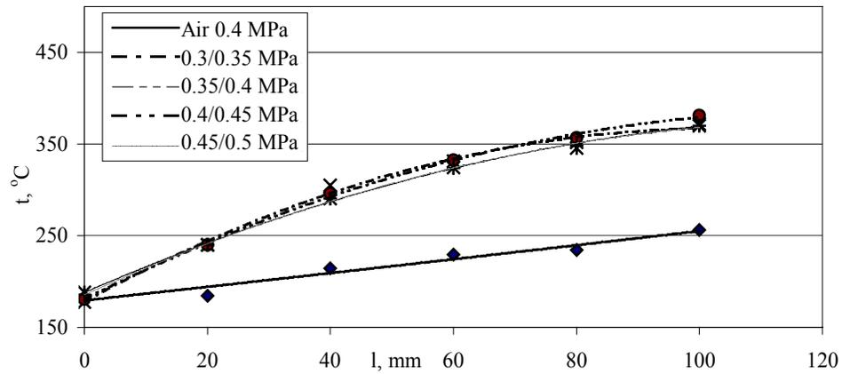
Fig. 8. Effect of distance from cooling nozzle axis and of cooling factor kind on temperature of casting die with cylindrical socket in heat transfer surface
