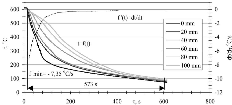
Fig. 5. Effect of time and distance from cooling nozzle axis on temperature and cooling rate with water mist under pressure 0.30/0.35 MPa of casting die with flat heat transfer surface
