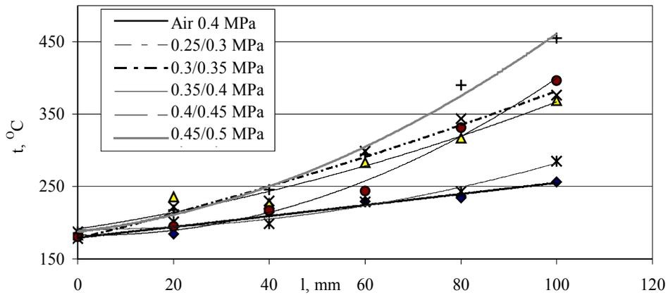
Fig. 7. Effect of distance from cooling nozzle axis and of cooling factor kind on temperature of casting die with flat heat transfer surface
