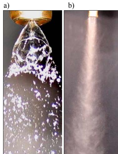
Fig. 3. Streams of sprayed water (a) and the water mist (b) cooling casting die surface with use of designed rotary sprayer, magnification of a) - x 3
