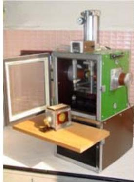
Fig. 5. Stand for ultrasonic testing of moulding sands
