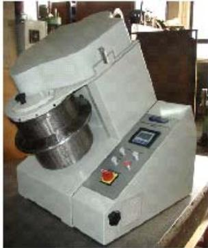
Fig. 4. Laboratory turbine mixer
