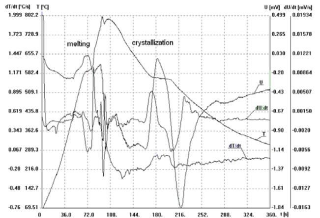
Fig. 4. Curves of ATND melting and crystallization of the alloy no. 2
