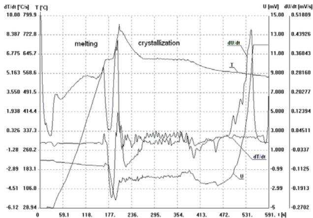
Fig. 3. Curves of ATND melting and crystallization of the alloy no. 1
