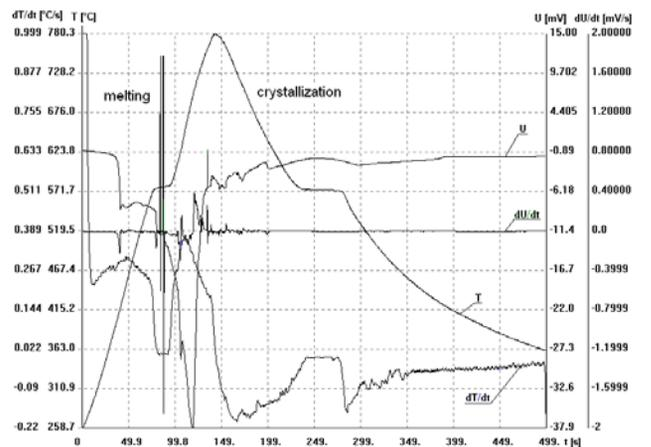
Fig. 5. Curves of ATND melting and crystallization of the alloy no. 3
