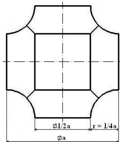
Fig. 3. Proportion of skeleton cell dimensions assumed for preparation of cast steel skeleton (substrate)
