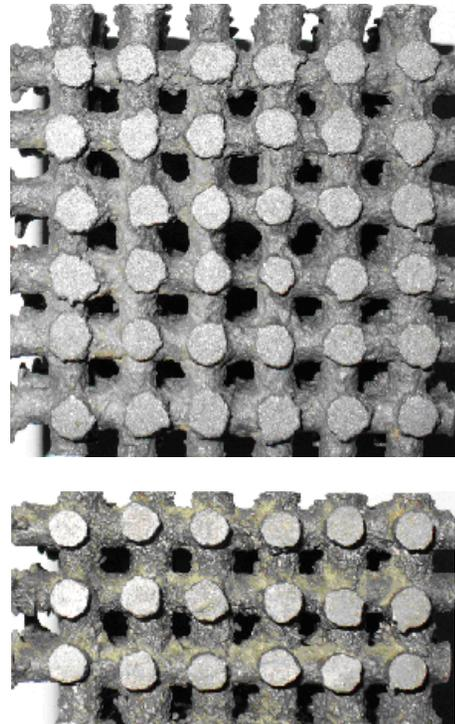
Fig. 5 Geometry of experimental skeleton castings made from cast steel
