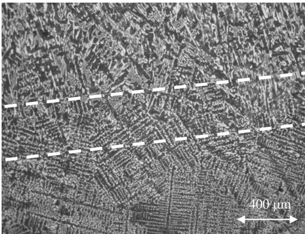
Fig. 6. Micrograph of cast iron structure showing structure refinement caused by heat flow kinetics in macroscale of bimetallic casting. Lines show boundary of transition between regions with different structure
