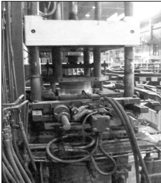
Fig. 1. Low pressure casting station of car wheels castings [2]
