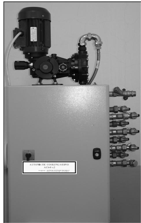
Fig. 2. Water mist cooling device [2]
