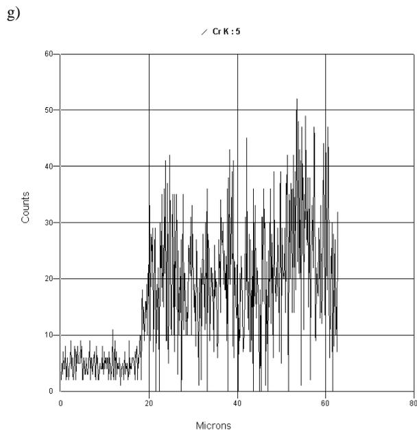
Fig. 5. The microstructure (a) and the linear distribution of: Si, Ni, Cu, C, Mo and Cr concentration (b ÷ g) within the eutectic grain
