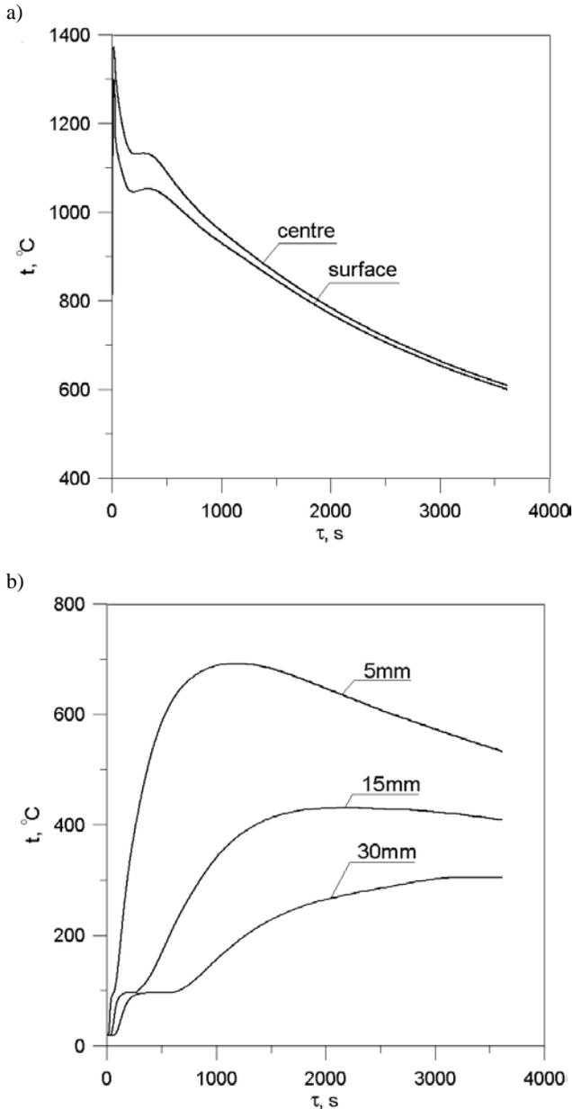
Fig. 1. Curves of cooling rate of the centre and surface of casting (a) and temperature change in moulding sand (b) at a distance of a: 5; 15 and 30mm from the surface of mould cavity
