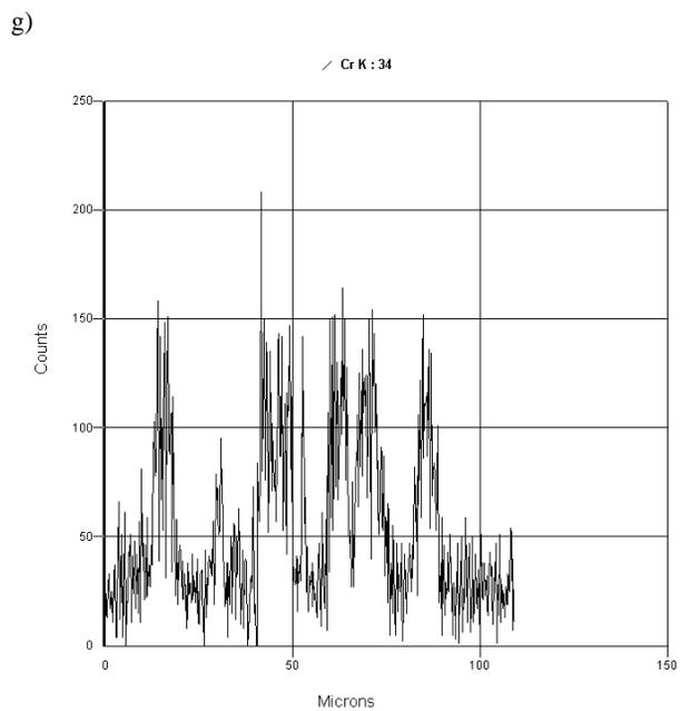
Fig. 4. The microstructure (a) and the linear distribution of: Si, Ni, Cu, C, Mo and Cr concentration (b ÷ g) within primary carbides
