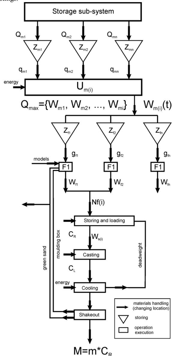
Fig. 1. Model of the process in the sand storage and preparation sub-systems
