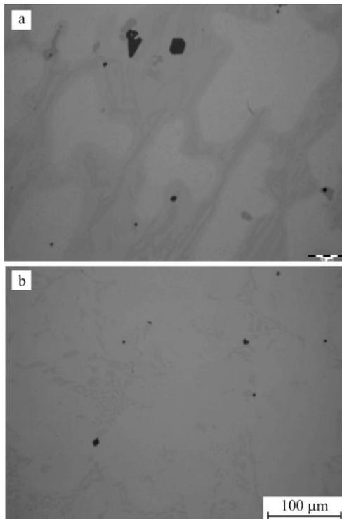
Fig. 7. Non-metallic inclusions in G-X40CrNiSi27-4 cast steel: a) in front of the filter, b) behind the filter; unetched state
