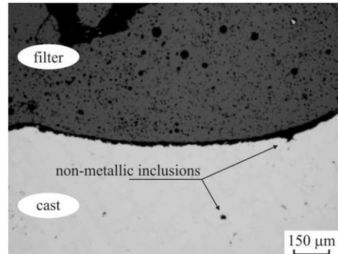
Fig. 8. Microstructure of GX40CrNiSi27-4 cast steel at the filter/metal interface; metallographic section; unetched
