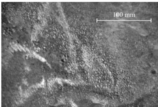
Fig. 2. Typical appearance of surface defects in cast hearth plates [2]
