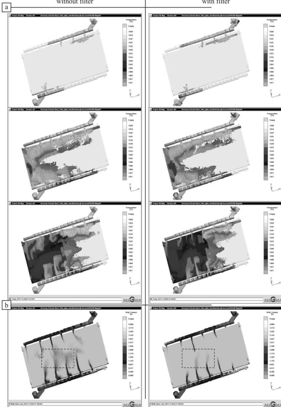
Fig. 5. The results of computer simulation of the mould cavity filling process when casting a hearth plate of 730×600 mm dimensions using the gating system without and with a 10 ppi filter [7]: a) temperature distribution on pouring, b) time necessary for molten metal to reach the top mould cavity; pouring temperature 1580°C, time of mould cavity filling through the gating system without filter – 30 seconds, and with filter – 35 seconds
