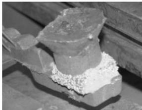
Fig. 4. Filter location in the gating system [7]
