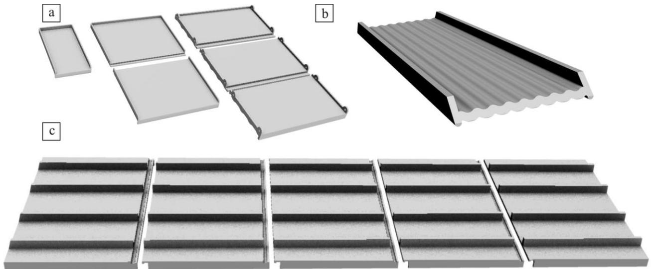
Fig. 1. Drawings of heat-resistant castings made by ZUT Foundry in Szczecin [2]: a) single- and multi-segment hearth plates, b) shaker plate, c) multi-segment plate for walking-hearth furnace
