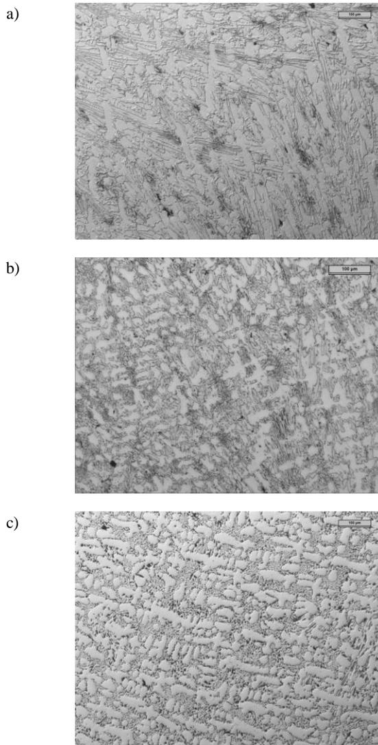
Fig. 1. Microstructures of castings made from high chromium cast iron: melt No 2 - (a), melt No 3 - (b), melt No 4 - (c)
