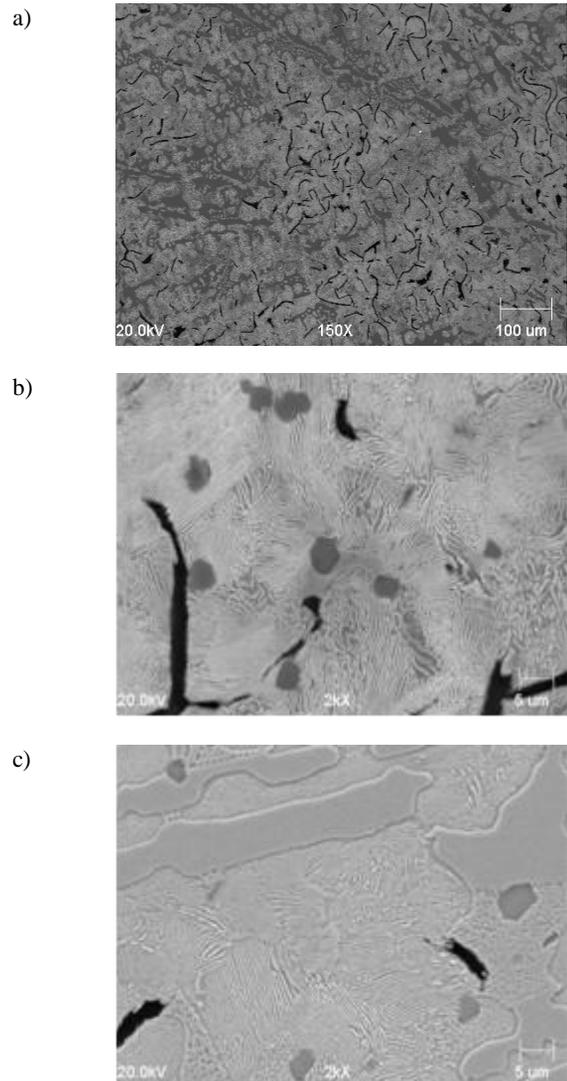
Fig. 3. Microstructures of castings made from low chromium cast iron at melt No 1 - (a) and aspect sulphides or phosphorus eutectic (steadyt) – (b, c)
