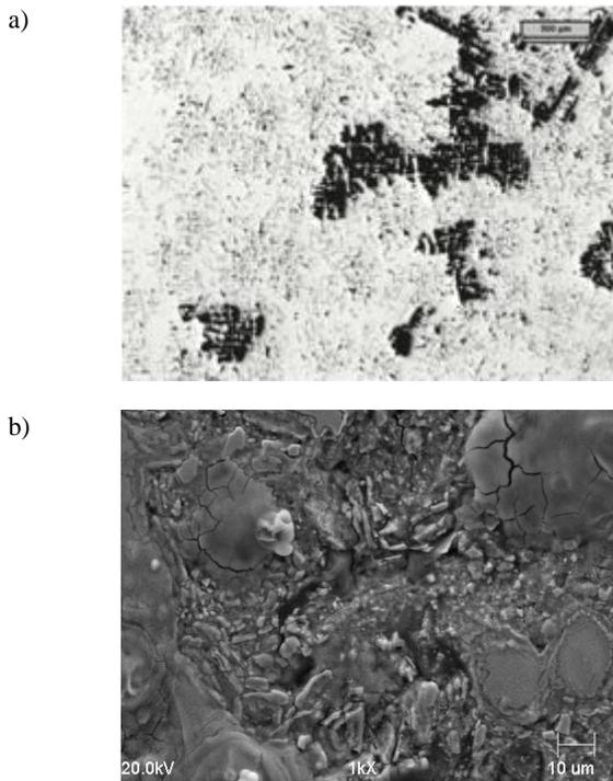
Fig. 4. Microstructures of castings made from low chromium cast iron at melt No 1 after heat treatment - (a) and microstructure SEM specific microareas (b)
