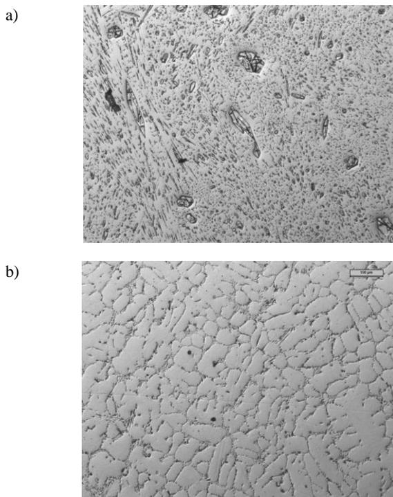
Fig. 2. Microstructures of castings made from high chromium cast iron: melt No 5 - (a), melt No 6 - (b)
