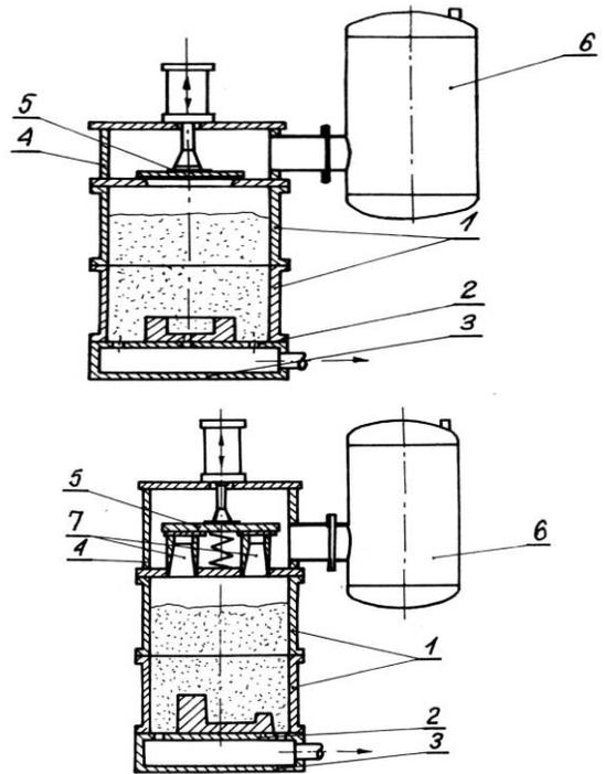
Fig. 4. Schematic diagram of forming lines patented by BMD [3], 1-moulding flasks, 2-vents, 3- vacuum chamber, 4- chamber, 5- valve, 6-pressure tank, 7- Level nozzle
