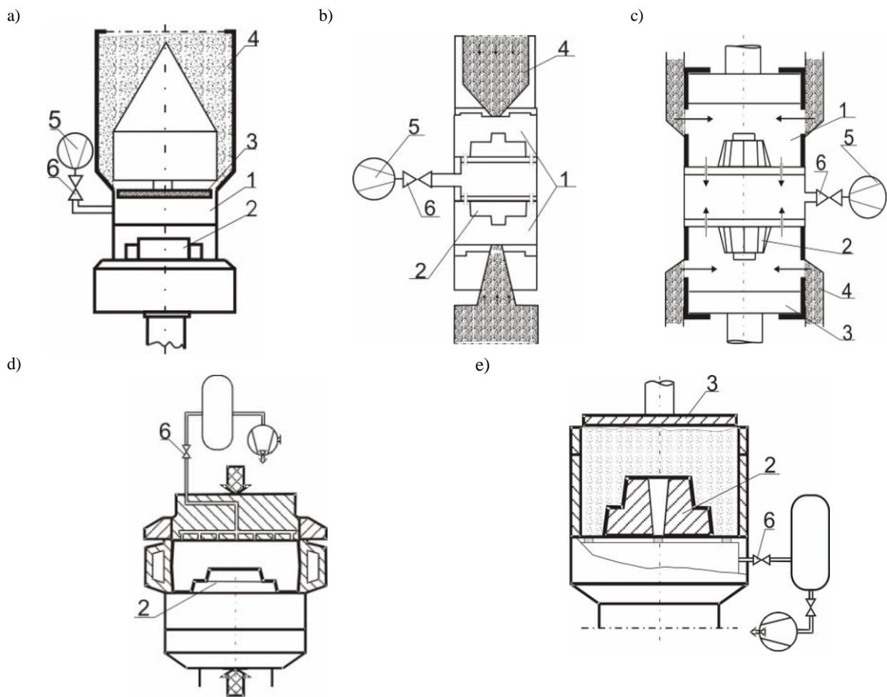
Fig. 5. Simplified diagrams of vacuum-assisted moulding systems [3, 8]: a)d) Kuenkel –Wagner- Vacupress version; b) Disa Forma; c) Haflinger; e) version of the process developed by the Authors;; 1- working space, 2- pattern plate, 3-pressing plate, 4- sand container; 5- vacuum installation; 6- valves
