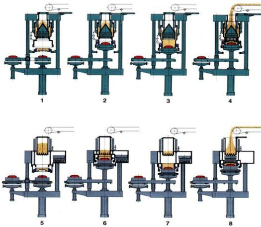
Fig. 1. Pressing machine Vacupress Kuenkel-Wagner [3]
