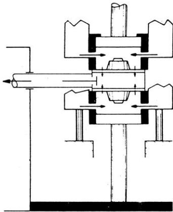
Fig. 2. Vacuum-assisted forming and pressing line (Haflinger) [3]
