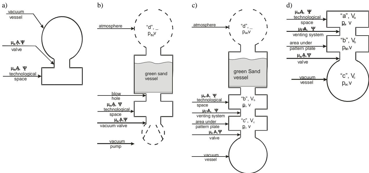
Fig. 6. Models of vacuum- assisted forming system corresponding to the structural diagrams: a & b) Kuenkel-Wagner (Fig 5 a, d); c) DISA Format (Fig 5 c); d) model developed by the Authors (Fig 5e)
