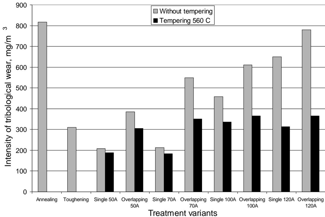
Fig. 4. Comparison of the intensity of tribological wear of the high speed steel HS 6-5-2 for different treatment variants
