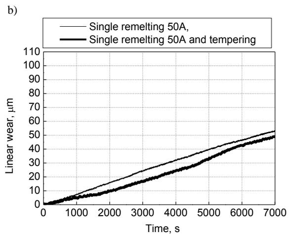
Fig. 2. Friction coefficient graph a) and linear wear b) in friction time function for the steel with single remelting with the amperage of 50A, before and after tempering in the temperature of 560°C
