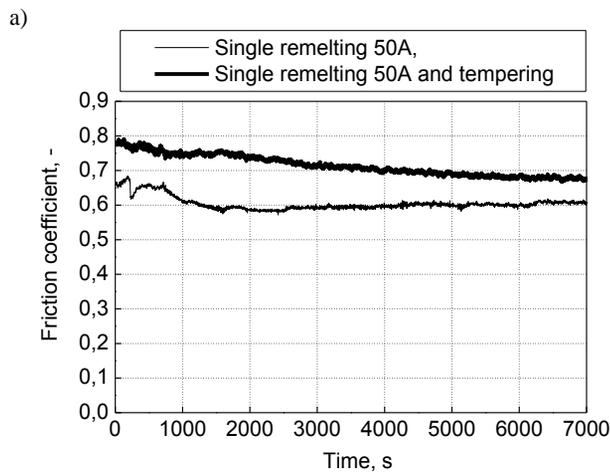
The Fig. 2 presents the graph of the friction coefficient and linear wear in the friction time function for the steel with the single remelting with the amperage of 50A before and after tempering in the temperature of 560°C.
