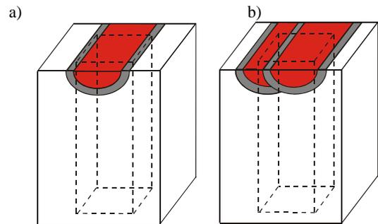
Fig. 1. The way of sample cutting for the tribological research; a) samples from single remelting, b) samples from the overlapping remeltings
