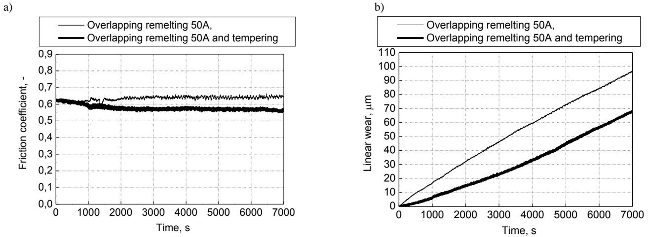
Fig. 3. The graph of friction coefficient a) and linear wear b) in friction time function for the steel with overlapping remeltings received for the amperage of 50A, before and after tempering in the temperature of 560°C
