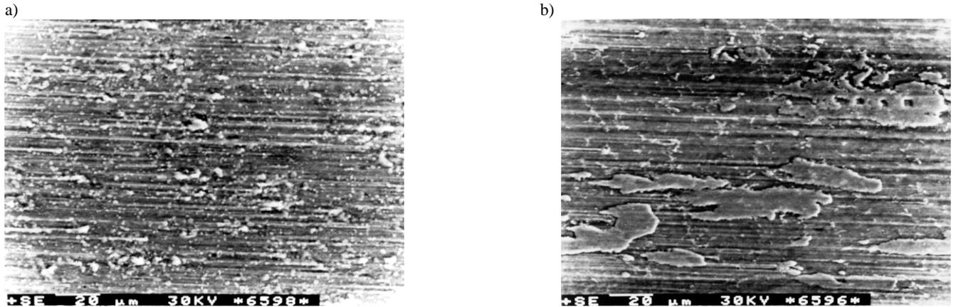
Fig. 5. The SEM view of the friction area of the samples made of the steel HS 6-5-2 remelted with the electric arc and tempered; a) the abrasion wear, b) the abrasion and adhesive wear
