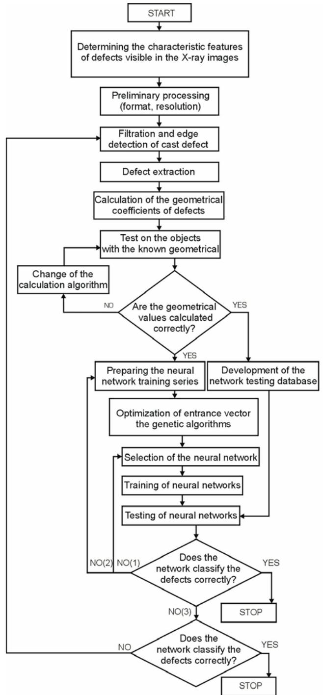
Fig. 2. Block diagram of the developed methodology of data processing pertaining to casting defects observed in the examined castings of the internal combustion engine elements from the Al-Si-Cu alloy
