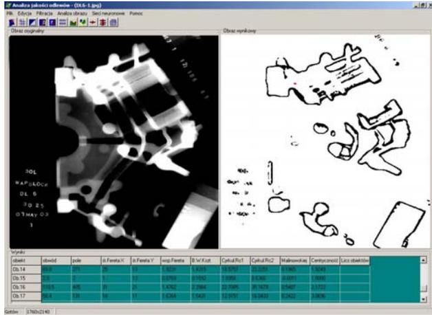
Fig. 3. The program window for the assessment of casting defects class
