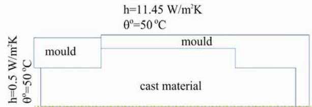
Fig. 1. Geometry of the system subjected to calculations of the temperature field within a roll and applied boundary conditions.
