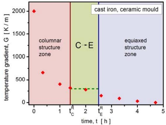
Fig. 8. Changes of the thermal gradient during solidification observed at the s/l interface: first, at the tips of columnar dendrites / cells, next at a layer of the equiaxed grains.
