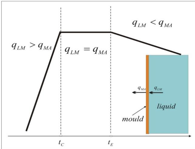
Fig. 3. Changes of temperature in function of time at the operating point situated in the ceramic mould; a/  $\dot{T} \gg 0$ , for  $t < t_C$ , b/  $\dot{T} = 0$ , for  $t_C < t < t_E$ , c/  $\dot{T} < 0$ , for  $t > t_E$ ;  $q_{LM}$  - heat flux from the liquid into the mould;  $q_{MA}$  - heat flux from the mould into the air.
