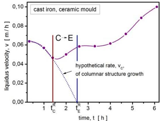
Fig. 9. Extrapolation of the columnar growth velocity to determine the time,  $t_E^R$ , that defines a full vanishing of the columnar structure.
