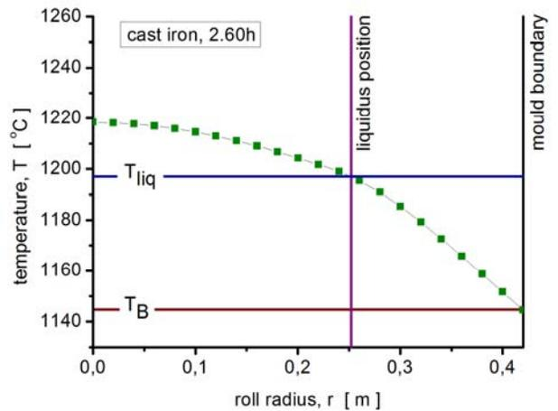
Fig. 6. Temperature field calculated for the time equal to 2.6 [h] within the cast iron roll of the 950 [mm] in diameter.
