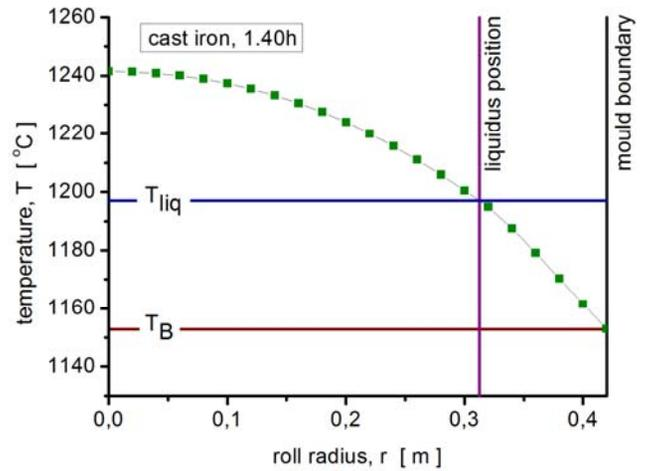
Fig. 4. Temperature field calculated for the time equal to 1.4 [h] within the cast iron roll of the 950 [mm] in diameter.
