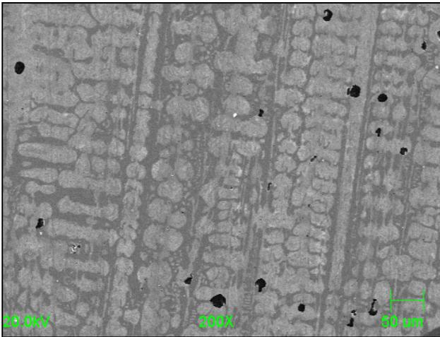
Fig. 10. Columnar structure as observed within the zone – C of the cast iron roll; nodular small particles of the graphite (black) are situated inside the austenite grains (bright).
