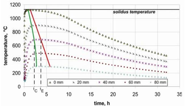
Fig. 2. Changes of temperature in function of time at different points situated in the mould as calculated for a given cast iron roll.
