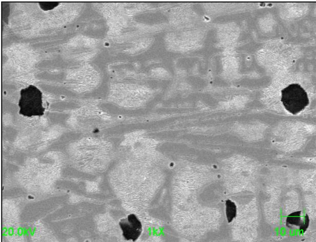
Fig. 11 Equiaxed structure (austenite and cementite) as observed within the zone – E of the cast iron roll; nodular small particles of the graphite (black) are situated inside the austenite grains (bright); nodular large particles of the graphite are also visible.
