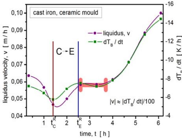
Fig. 7. Velocity of the *liquidus* isotherm movement in function of time; additionally  $dT_B / dt$ , as observed at the roll / mould border is shown; the  $t_C^R \leftrightarrow t_E^R$  period of time is distinguished.
