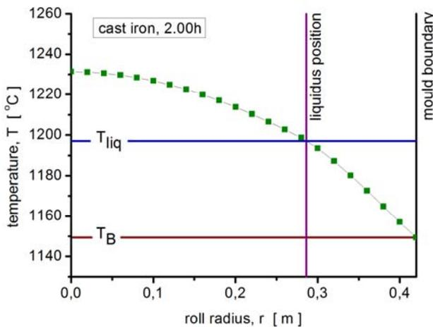
Fig. 5. Temperature field calculated for the time equal to 2.0 [h] within the cast iron roll of the 950 [mm] in diameter.
