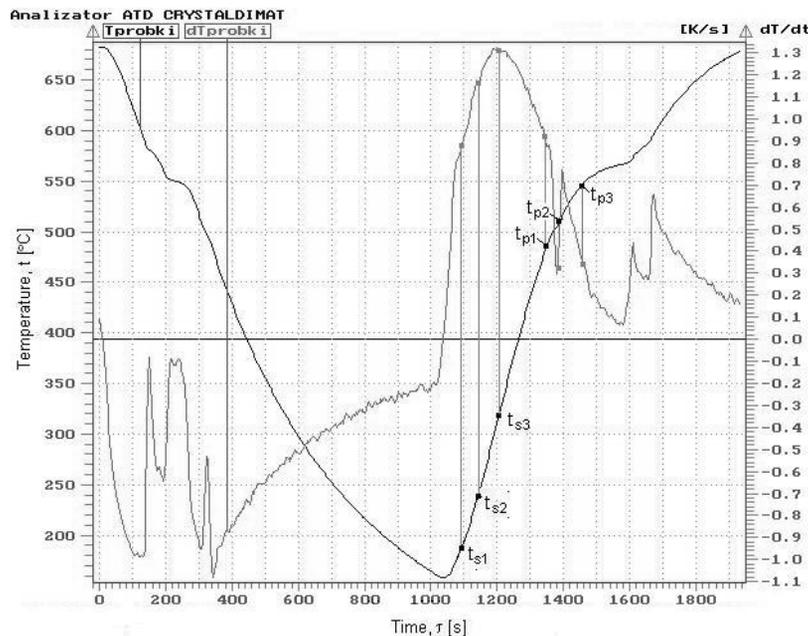
Fig. 1. Curves of the ATD method for refined and modified EN AC-46000 alloy
