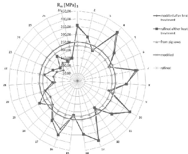
Fig. 2. Change of  $R_m$  tesile strength of the investigated alloy for individual configurations of the testing plan
