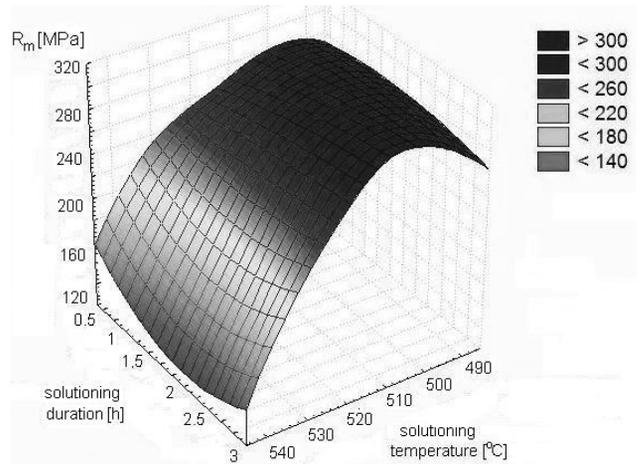
Fig. 3. Effect of temperature and duration of solutioning on  $R_m$  tensile strength of the EN AC-46000 alloy
