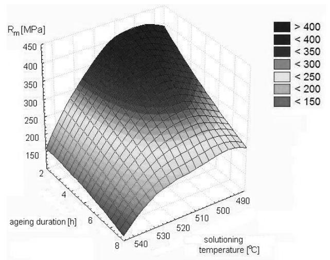
Fig. 4. Effect of temperature solutioning and duration ageing on  $R_m$  tensile strength of the EN AC-46000 alloy
