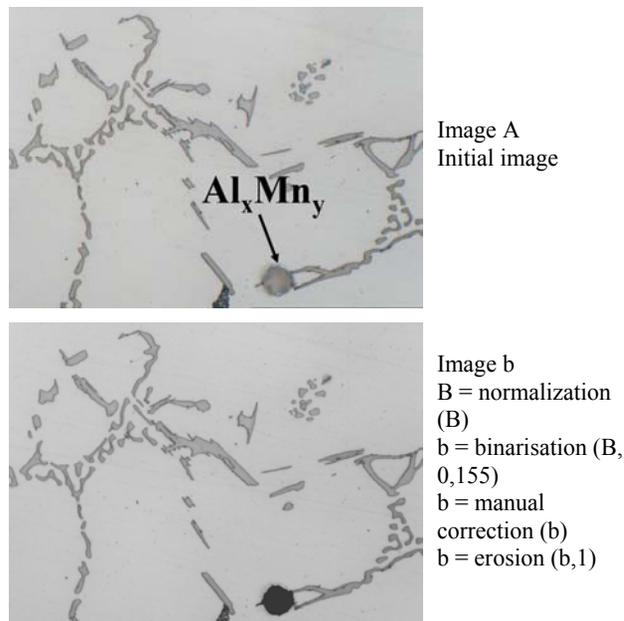
Fig. 6. Semi-automatic procedure used to detection of Al-Mn compound.
