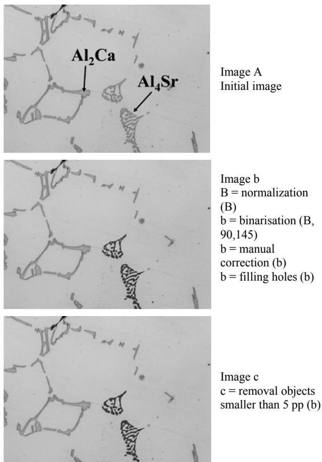
Fig. 4. Semi-automatic procedure used to detection of  $\text{Al}_4\text{Sr}$  phase.
