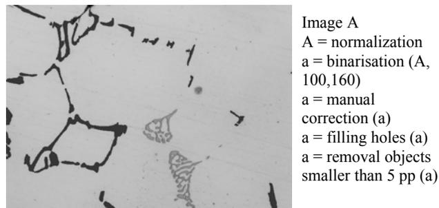
Fig. 5. Semi-automatic procedure used to detection of  $\text{Al}_2\text{Ca}$  phase.
