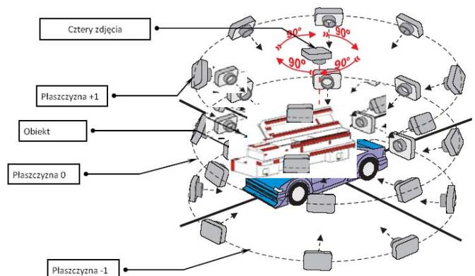
Fig. 3. Measurement Strategy C. Application of the photogrammetric system for the identification of the coded and non-coded reference points
