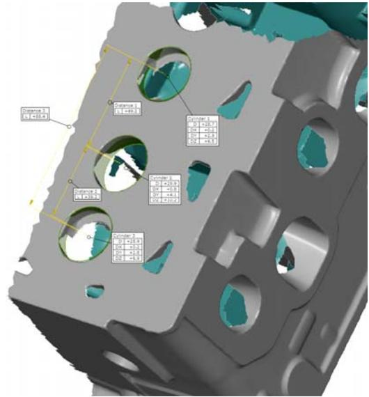
Fig. 6. Example of the measurement results for the characteristics of geometrical features (diameters of the orifices, their localization and distances between them in the defined coordinate system)
