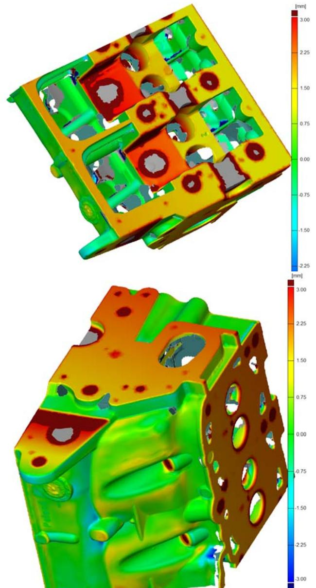
Fig. 8. Distribution of the deviations (values of the allowances) in the best-fitting simulation
