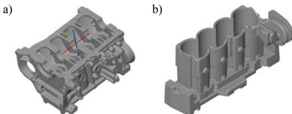
Rys. 5. A picture of an engine block (a) and core (b) obtained with ATOS [courtesy of GOM]
