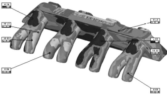
Fig. 7. Measurement result of core at inlet core of cylinder head
