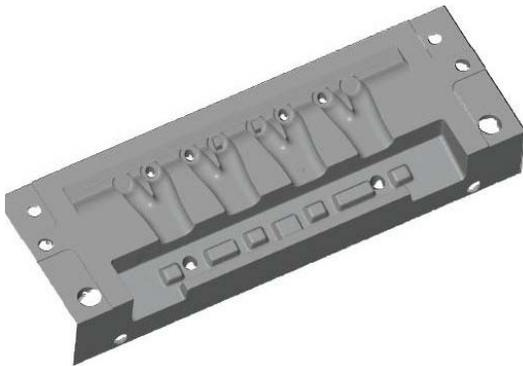
Fig. 9. Tool image after measurement with ATOS GOM
