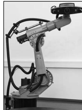
Fig. 6. ATOS head on robot arm
