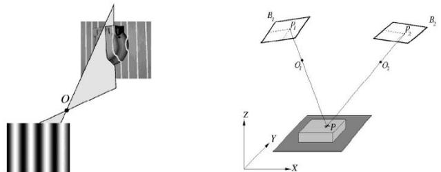
Fig. 3. Fringes projection and triangulation
