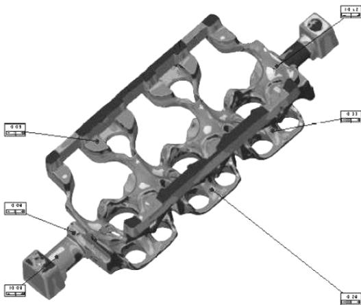
Fig. 8. Measurement result of core at water core of cylinder head
