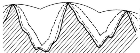
Fig. 2. An outlook of profile measured with different tip radii: 1 - solid line shows pickup with 10  $\mu m$  radius, 2 - short segmented line stands for pickup with 5  $\mu m$  radius, 3 - line with segments and points stands for pickup with 2  $\mu m$  radius.
