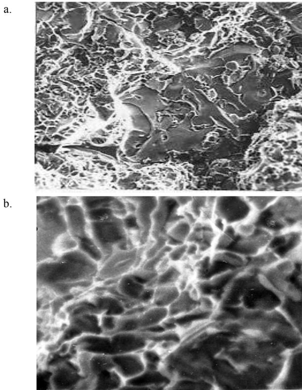
Fig.2. The fracture surface of impact tested specimens No 8 taken at different magnification: a – x1000 and b – x5000
