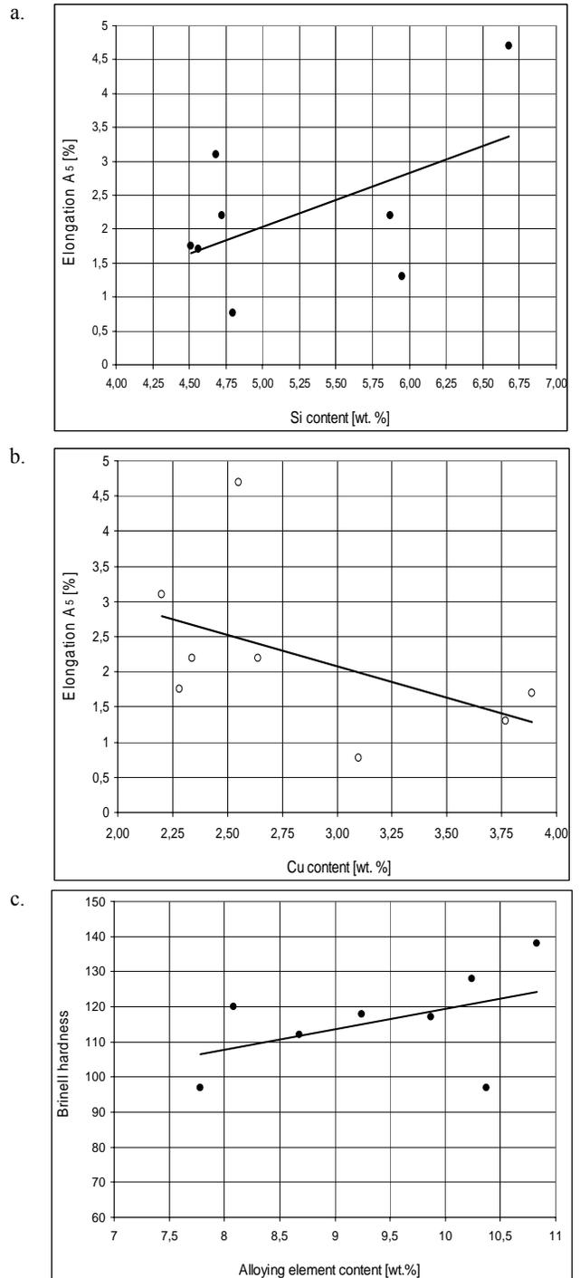
Fig.7. The dependence of ductility on: a – Si and b – Cu; c – the influence of total alloying elements content on Brinell hardness
