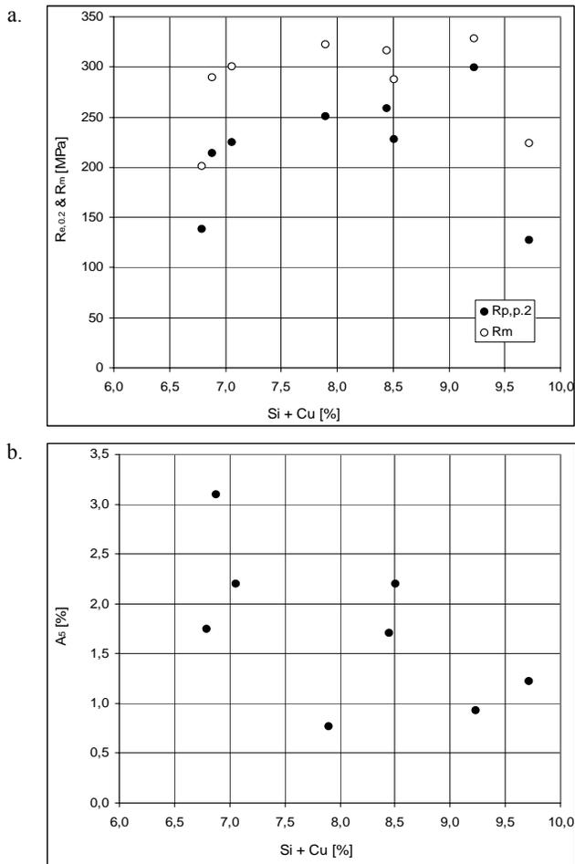
Fig.6. The influence of main alloying elements on: a -  $R_{e, 0.2}$  and  $R_m$  values and b -  $A_5$
