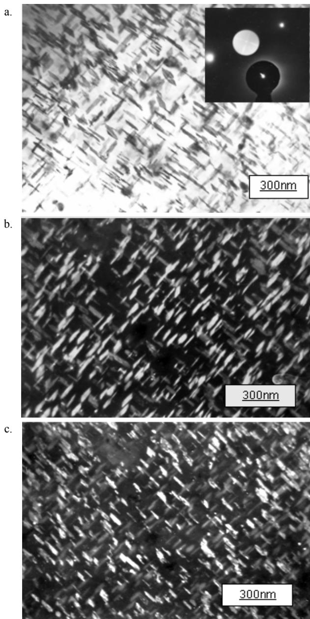
Fig.4. The structure AlSi5Cu3(Mg) type alloy - No4: a – bright-field, b and c – dark-field micrographs taken from two opposite reflexes, one of which is marked in selected area diffraction pattern (SAD) showed in right corner fig.4a
