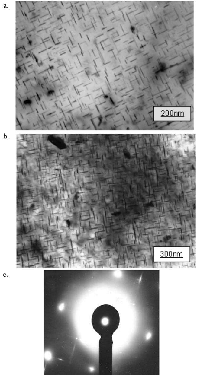
Fig.3. An electron micrographs of age hardened AlSi5Cu3(Mg) type cast alloys: a – No 1 (x45.000), b – No 2 (x40.000) and c – SAD from the area showed in fig 3b.
