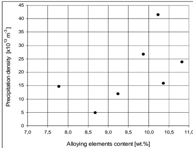
Fig.8. The density of precipitates as a function of alloying elements content
