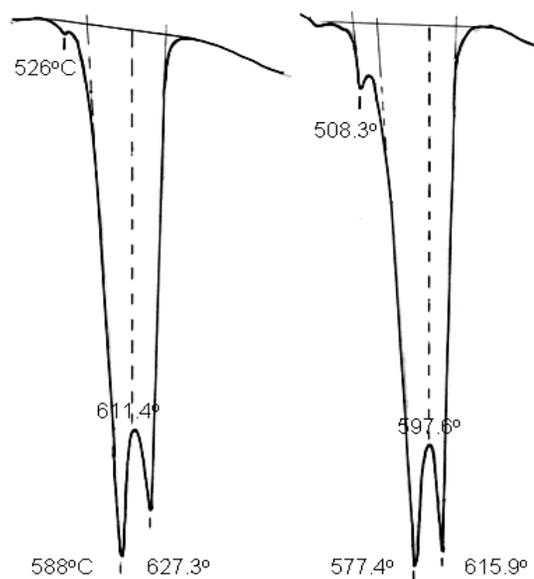
Fig.5. The example of DTA curve obtained for on of AlSi5Cu3(Mg) – type cast alloy studied in this elaboration
