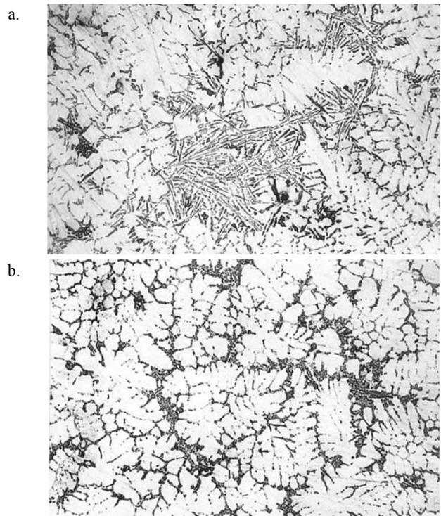
Fig.1. The microstructure AlSi5Cu3(Mg) alloy: a – alloy No 5 (Si + Cu = 9.23%) and b – No 8 (Si + Cu = 6.88%) (magn. x50)
