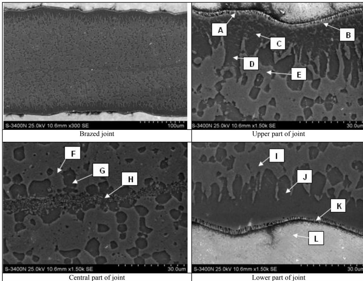
Table 9. Results of spectral chemical analysis (EDS) of phases in structures of joint made of alloy based on TiAl ( $\gamma$ ) intermetallic phase brazed with copper filler metal at 1050°C (denotation of phases corresponds to phases from Table 8)
