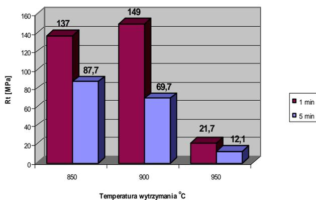
Fig. 4. Shear strength of TiAl48Cr2Nb2 alloy joints produced with B-Ag72Cu-780 filler metal foil
