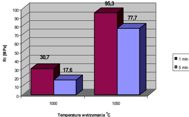
Fig. 3. Shear strength of TiAl48Cr2Nb2 alloy joints produced with Cu foil
