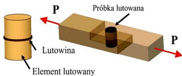
Fig. 2. Sample for static shearing test
