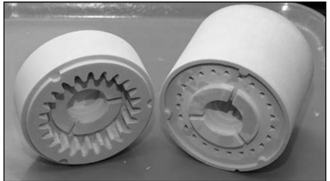
Fig. 3. The casting form after infiltration
