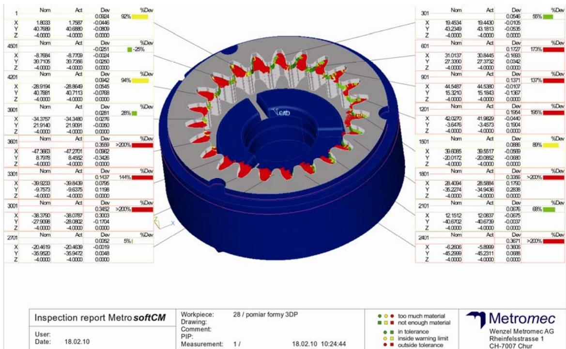
Fig. 5. Protocol of toothed wheel rim form measurement
