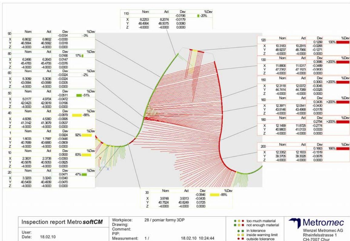
Fig. 6. Detailed protocol of tooth profile measurement
