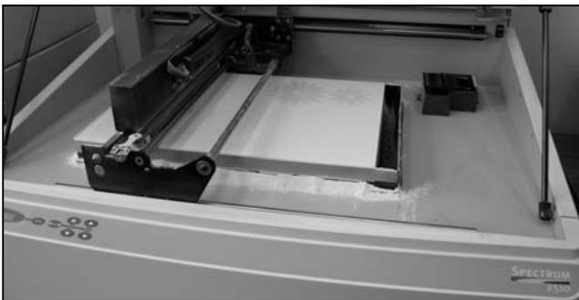
Fig. 2. 3D Z510 Spectrum printer while working
