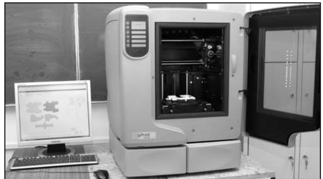
Fig. 12. RP FDM U-Print device
