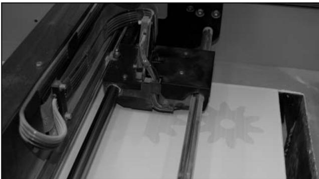
Fig. 6. Print out of model layer by 3DP method – Z510 Spectrum printer
