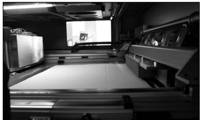
Fig. 8. Layer application in VoxelJet device chamber
