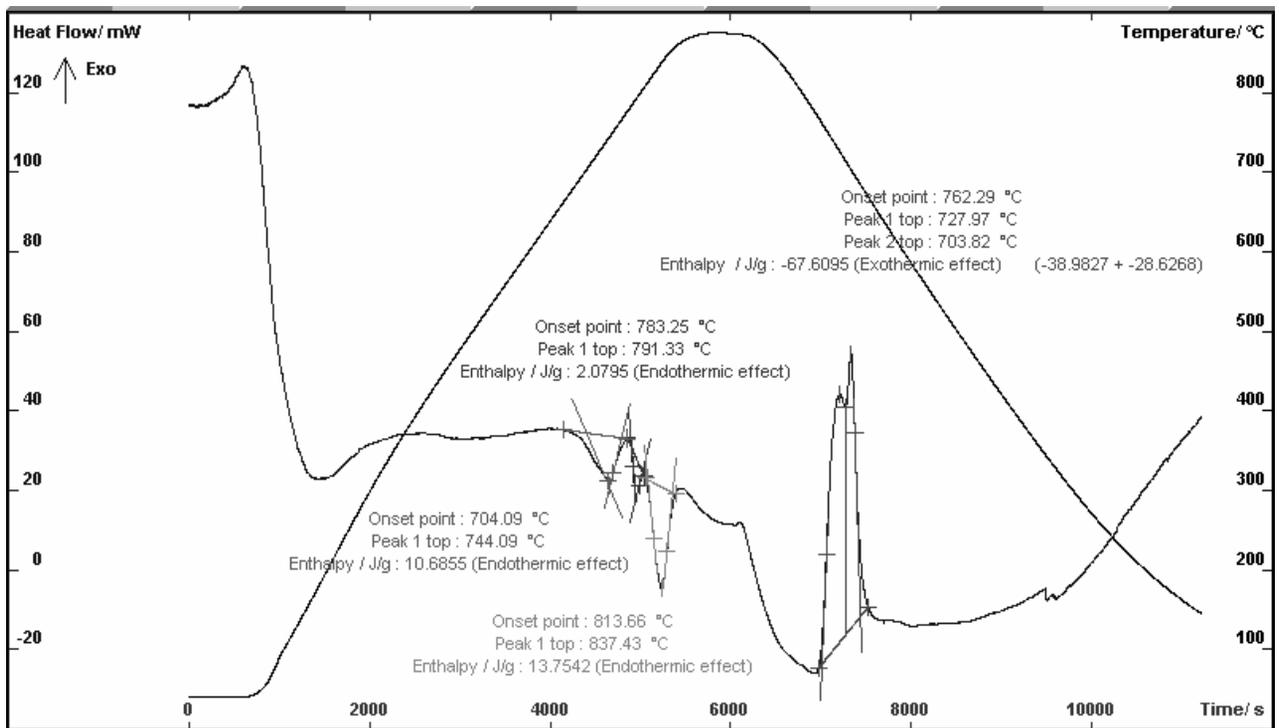
Fig. 3. The DSC diagram of nodular cast iron heating and cooling – casting wall 5 mm thick
