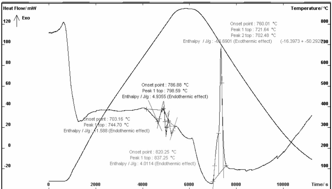
Fig. 4. The DSC diagram of nodular cast iron heating and cooling – casting wall 20 mm thick
