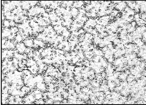
Fig. 1. Microstructure of AZ91 alloy ingot
