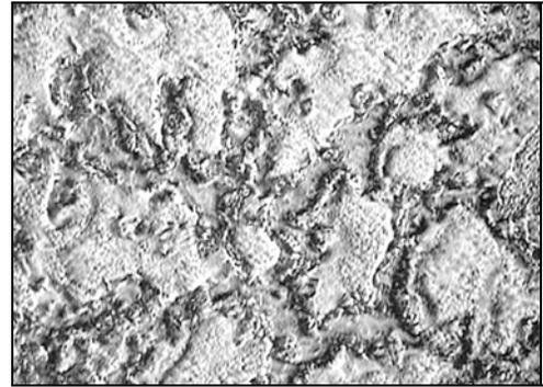
Fig. 4. Microstructure of a pressure casting made of remelted AZ91 alloy ingot
