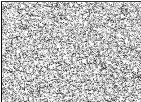
Fig. 3. Microstructure of a pressure casting made of metal containing 30% of AZ91 alloy home scrap
