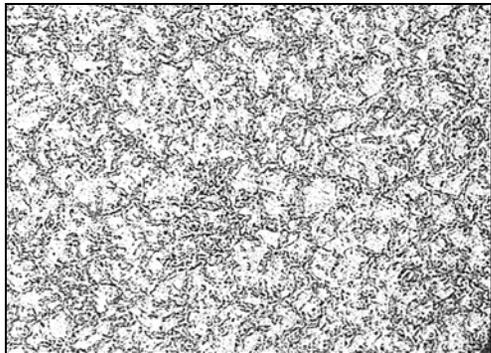
Fig. 2. Microstructure of a pressure casting made of remelted AZ91 alloy ingot
