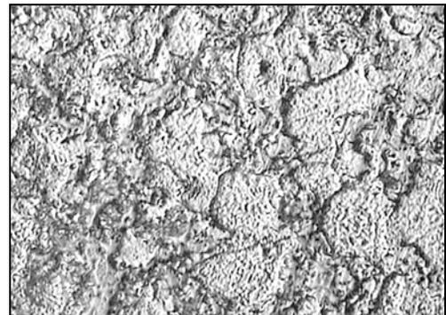
Fig. 5. Microstructure of a pressure casting made of metal containing 30% of AZ91 alloy home scrap
