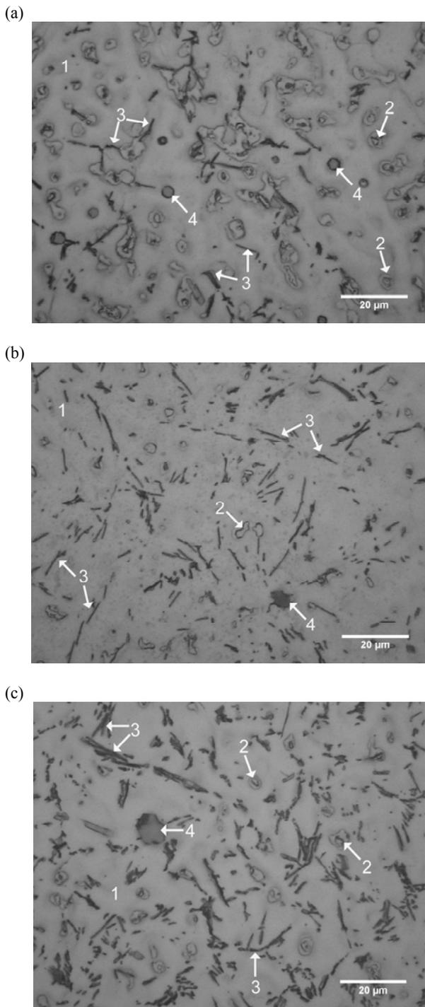
Fig. 2. Microstructure of as-cast a) AM50+1%RE, b) AM50+2%RE, c) AM50+3%RE alloys; LM
