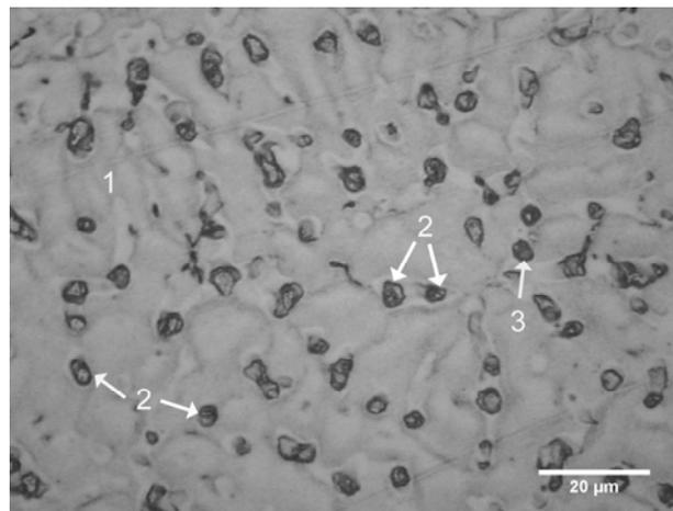
Fig. 1. Microstructure of as-cast AM50 alloy; LM
