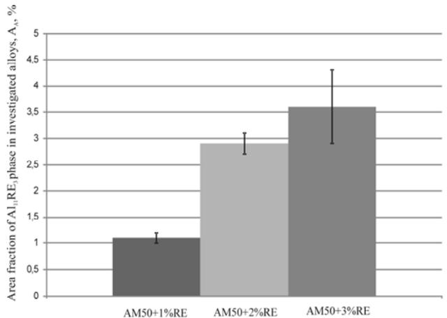
Fig. 4. Influence of RE addition on the area fraction of  $Al_{11}RE_3$  phase in investigated alloys
