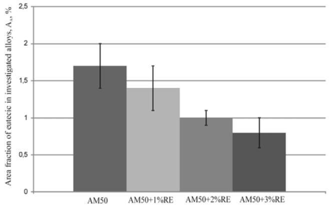
Fig. 3. Influence of RE addition on the area fraction of eutectic in investigated alloys
