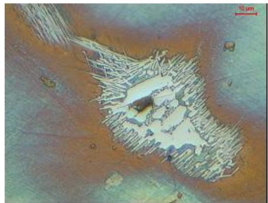
Fig. 10. Cast high manganese steel, before the heat treatment
