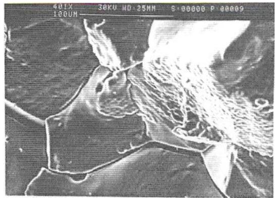
Fig. 5. Intergranular, brittle fracture formed at 1275 °C
