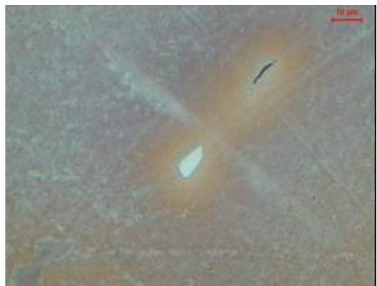
Fig 13. Carbides in high manganese steel after 10h at 1050 °C and water quenched. Solidification modulus of casting 9 cm
