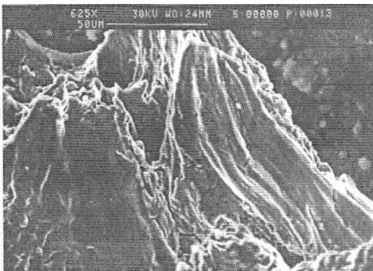
Fig. 8. Sample tested at 1131 °C. High plastic deformation
