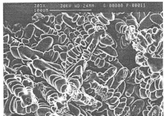
Fig. 9. The free dendrites in axial zone (porosities)
