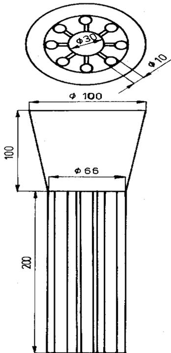
Fig. 1. Test sample for high manganese steel
