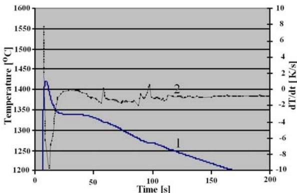
Fig. 2. Cooling Curve of high manganese steel. 1 – temperature, 2- derivative of temperature.
