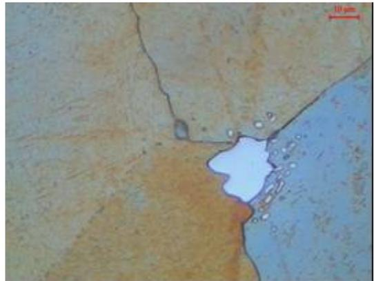
Fig. 11. Carbides in high manganese steel after 3h at 1050 °C and water quenched. Solidification modulus of casting 9 cm
