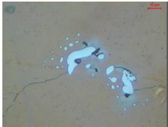
Fig. 12. Carbides in high manganese steel after 5h at 1050 °C and water quenched. Solidification modulus of casting 9 cm
