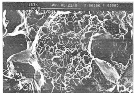
Fig. 7. The axial zone of sample with the porosities
