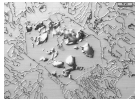
Fig. 4. The primary carbide precipitate (Cr, Fe)_7C_3
