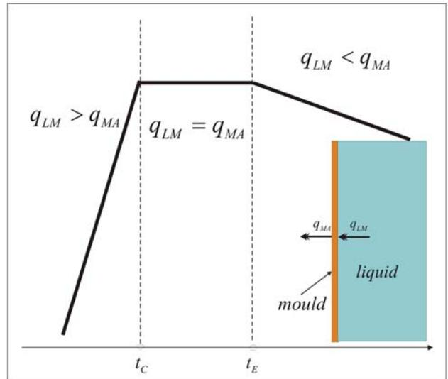
Fig. 4. Scheme of temperature field versus time for an operating point defined in Fig. 2, (casting steel): a/ below  $t_C$ ,  $\dot{T} \gg 0$ , b/ within  $t_C \leftrightarrow t_E$ ,  $\dot{T} = 0$ ,  $\partial T / \partial r|_{t_C} \approx \partial T / \partial r|_{t_E}$ , (Fig. 3), for all values of roll radius, and c/ above the time  $t_E$ ,  $\dot{T} < 0$ . The interplay between heat fluxes ( $q_{LM}$  liquid → mould and  $q_{MA}$  mould → air) described for three discussed time periods
