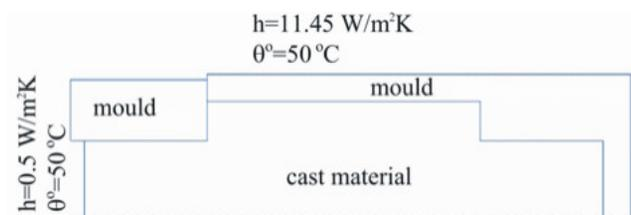
Fig. 1. Geometry of temperature field (for a roll) and applied boundary conditions
