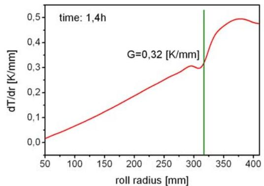
Fig. 7. Temperature gradients versus roll radius. Vertical line denotes the position of liquidus temperature. The temperature gradient at the tip of growing columnar dendrite is  $G = 3.2$  [K/cm]
