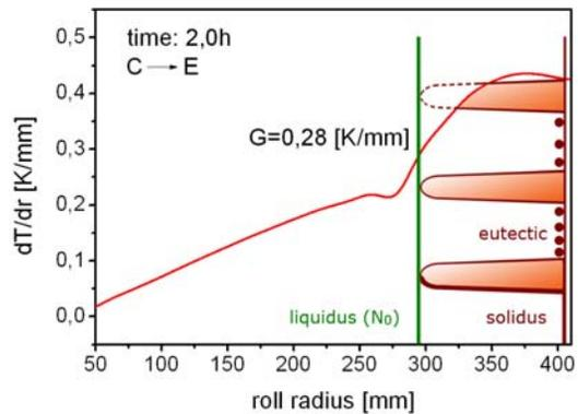
Fig. 11 Temperature gradients versus roll radius. Vertical lines denote the positions of liquidus and solidus temperature, respectively.
