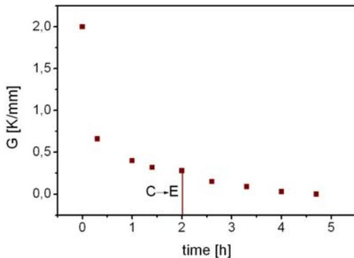
Fig. 9. Temperature gradient calculated for the tips of growing dendrite (for  $liquidus(N_0)$  versus time of roll solidification
