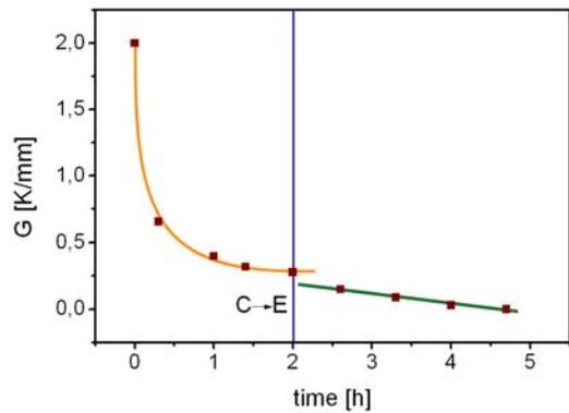
Fig. 10 Tendencies in the behavior of temperature gradients The boundary between tendencies indicates the time for  $C \rightarrow E$  transition.
