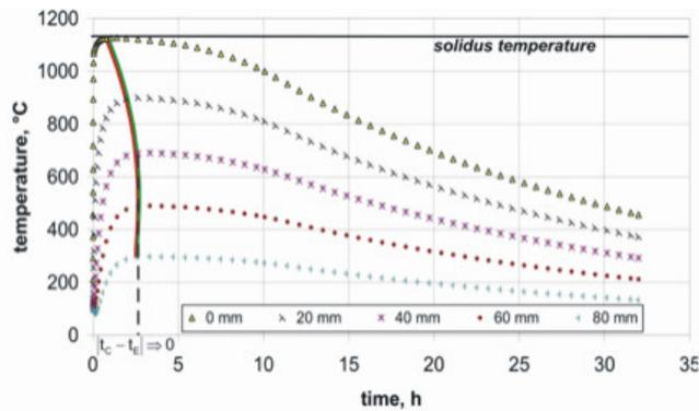
Fig. 5. Changes of temperature versus time at different points situated in the mould as calculated for a middle massive roll made of cast iron. Intersection of vertical curves with temperature profile printed for middle point of mould defines the period of time  $t_C \leftrightarrow t_E$
