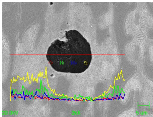
Fig. 13. Morphology of the eutectic grains (nodular graphite enveloped by austenite, dark areas–cementite, bright areas–austenite. Small particles of nodular graphite are also visible inside the dendrite
