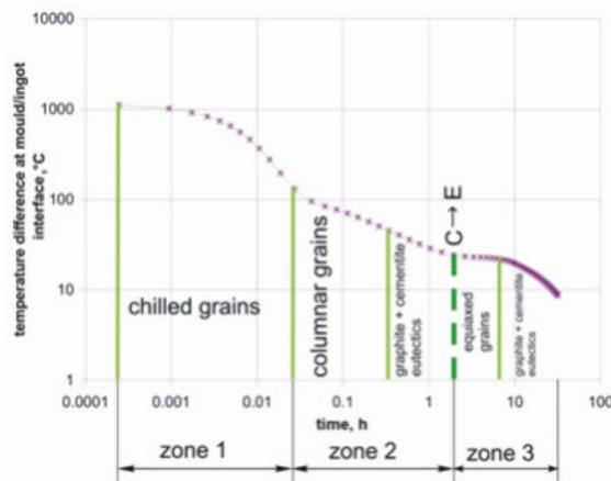
Fig. 6. Periods of time (distinguished zones) referred to the formation of different types of structure in the solidifying roll
