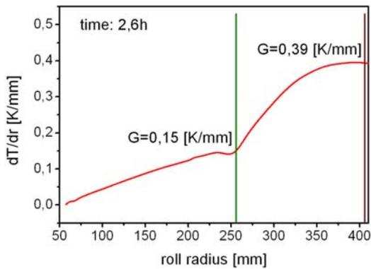
Fig. 8. Temperature gradients versus roll radius. Vertical lines denote the positions of liquidus and solidus temperature, respectively. The temperature gradient at the tip of growing columnar dendrite is  $G = 1.5$  [K/cm]
