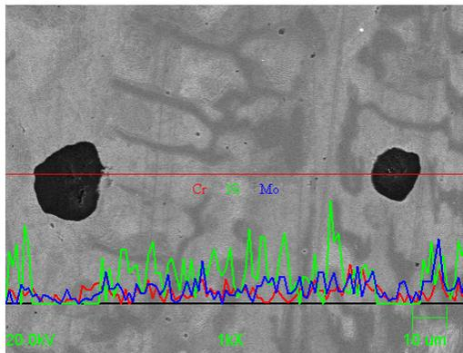
Fig. 12. Morphology of the cast iron roll revealed at 3 mm from the roll surface. Black particles – nodular graphite, dark areas – cementite, bright areas – austenite. Small particles of nodular graphite are also visible inside the dendrite. The phenomenon of graphite particles enveloping by austenite has been revealed and explained, [6-7]
